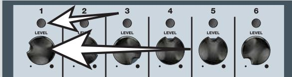
10. Set up each of the other channels in the same way. Use the channel Level knobs to adjust the relative loudness of each channel until you get the right overall balance, then use the master Volume knob to adjust everything together. The master Volume knob on your Passport has signal level meters. If you see the meters illuminate into the red zone, turn down the master Volume knob.
