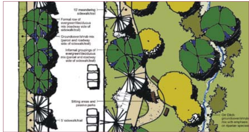
Figure 4-5. Sample Bufferyard Landscaping Requirements.
