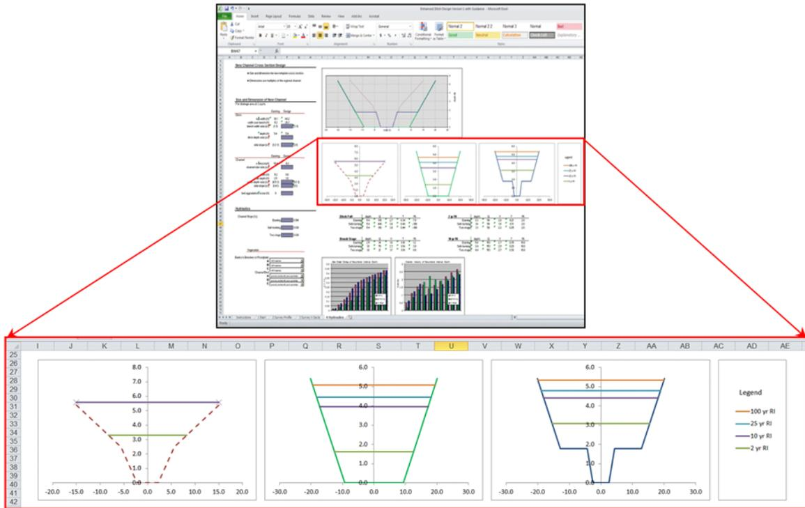
Figure 22. Estimated elevations of the water surface for the 2-, 10-, 25-, and 100-year storm events.
