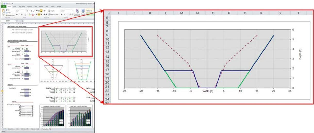
Figure 21. Overlay of channel geometries for the representative existing channel and the proposed two-stage and self-forming channels.
