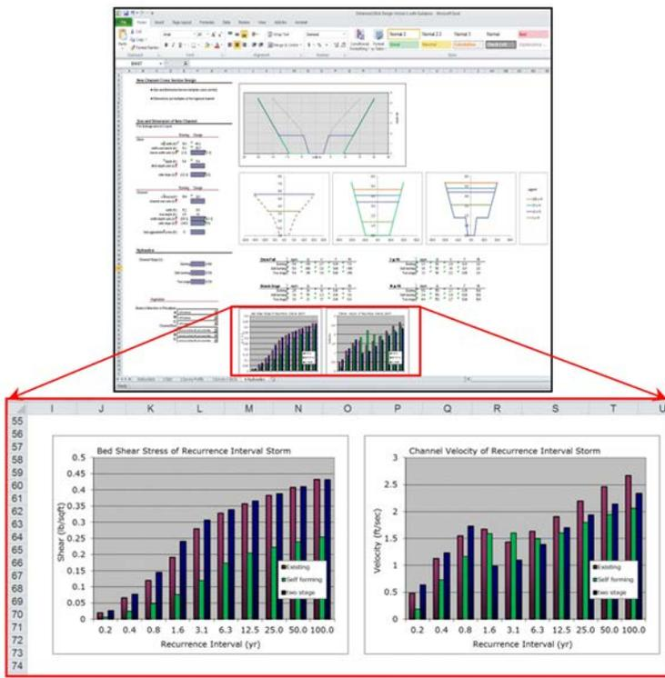
Figure 24. A comparison of channel velocities and bed shear stresses for the existing channel and the proposed two-stage and self-forming channels. Values are provided for a number of frequent and infrequent flow events.
