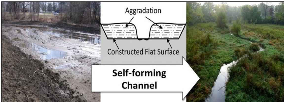
Figure 3. A self-forming channel.
