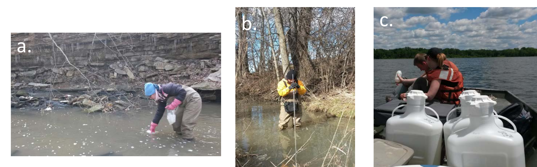
Figure 3. Water collection for nutrient analysis (a), measurement of streamflow velocity (b), and collection containers for \delta^{18}O phosphate samples (c).
