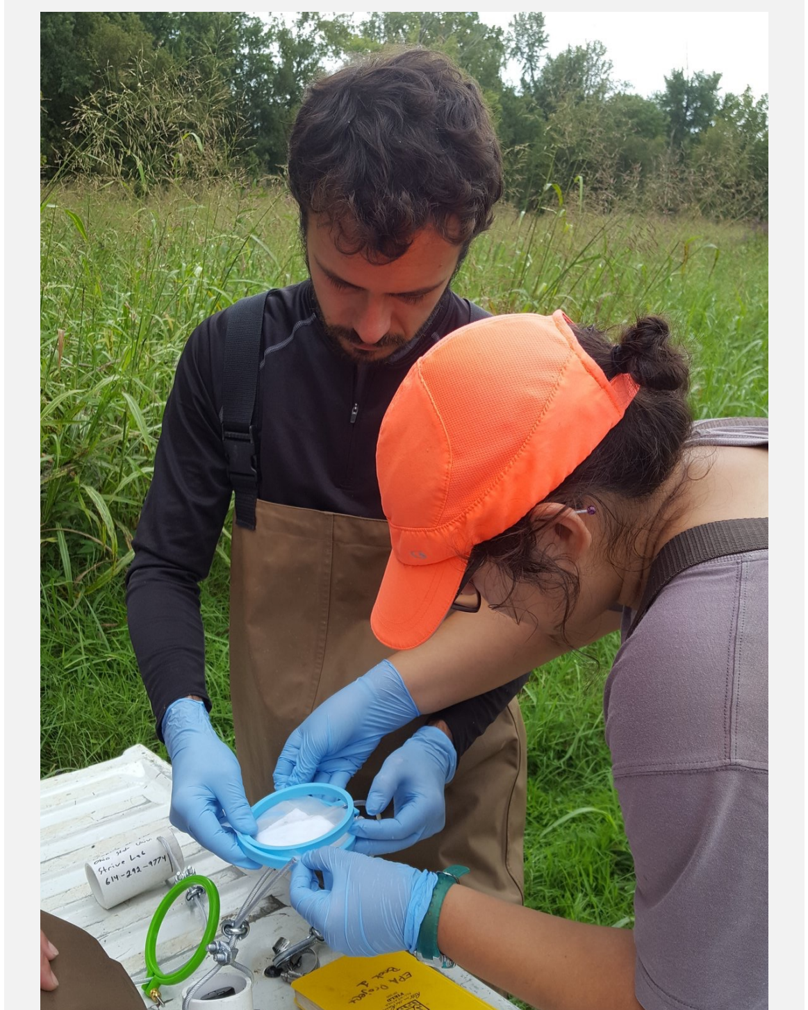
Figure 4. A SPATT sampler being prepared for deployment to measure cyanotoxins in streams.
