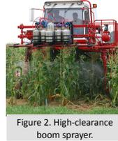
Figure 2. High-clearance boom sprayer.
