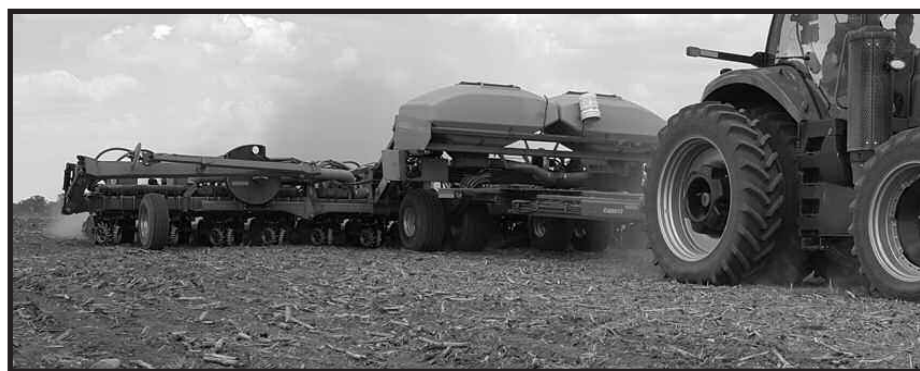
Planter tires in the center section can result in lower yields for the "pinch rows."
