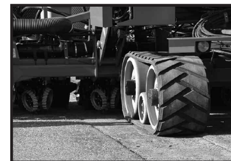
Rubber tracks can reduce pinch row compaction. However, in 2017 research, corn yields were statistically equal.
