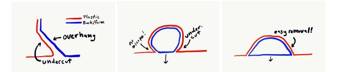
Risers - depending on the type and thickness of plastic you are using, plan to add a riser to the base of your mold. This will help avoid a bevel or fillet where the base of the buck meets the vacuum former platen.
