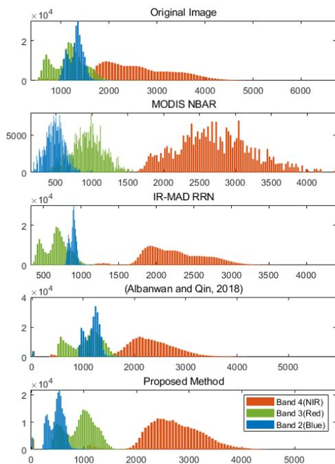
Fig. 6. The spectral analysis using the histograms for a sample of bands: NIR, Red, and Blue comparing the original image, MODIS's reference data, (Albanwan & Qin, 2018), IR-MAD, and our proposed method for region 2. All the figures share the same legend.
