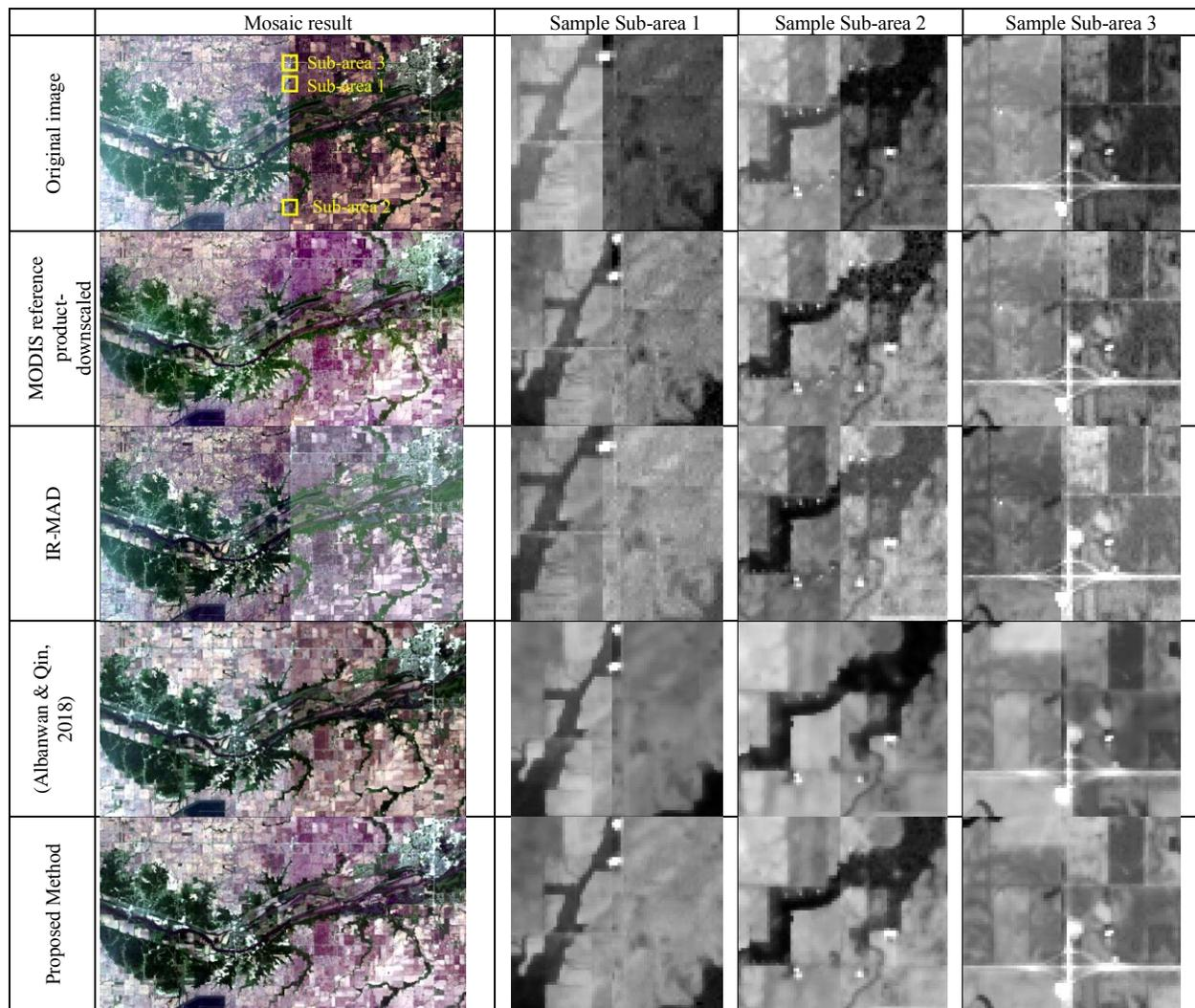
Fig. 4. A visual radiometric consistency comparison using a Mosaic before and after the normalization of region 1 in Time 1 and region 2 in Time 2. Note the image reflectance uses the same scaling so their visuals reflect the absolute reflectance. (RGB: Band 1, 2, 3(Landsat-7 ETM+)/Band 2, 3, 4(Landsat 8/OLI)).
