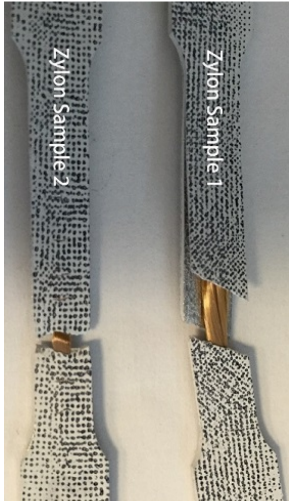
Figure 2.39: PBO Sample 1 and 2, post testing.
