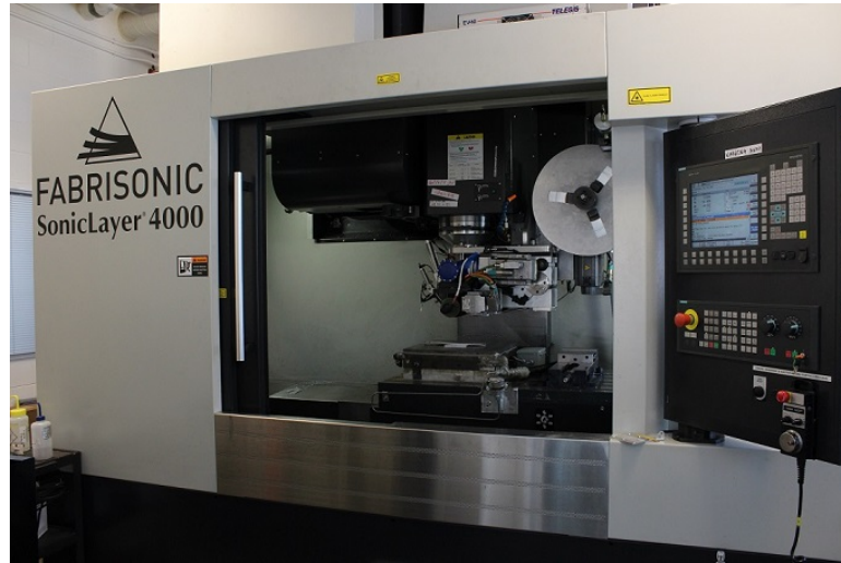
Figure 1.2: Fabrisonic's SonicLayer ® 4000, Ohio State University's UAM machine.
