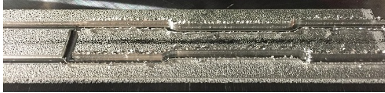
Figure 2.21: SiC embedded dog-bone with rough edges due to dulling of end-mill as part of the machining process.
