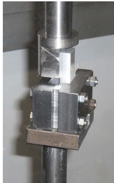
Fig. 5 UAM shear specimen strength testing set-up
