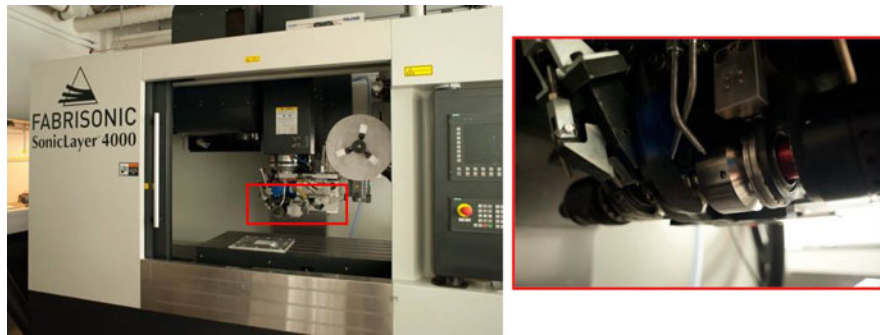
FIG. 3. UAM system at Ohio State University, with close up view of the ultrasonic assembly.
