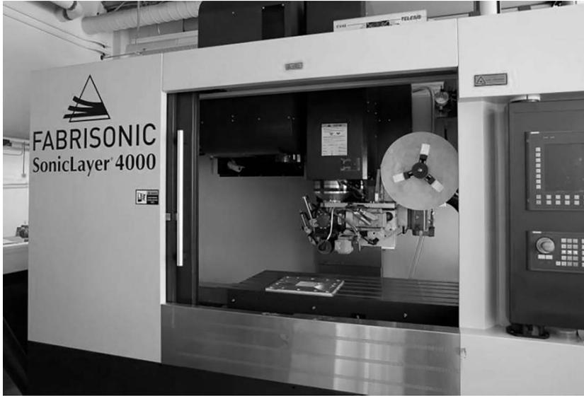
**Figure 17.3** (See color insert.) State of the art UAM system featuring a 9 kW welder and 20 kN of normal force. This amount of power makes it possible to make high quality, gapless metallic parts.
