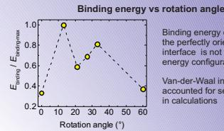
Binding energy calculations show the perfectly oriented GaAs/graphene interface is not the minimum energy configuration
