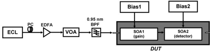
Fig. 6. SOA gain measurement setup
