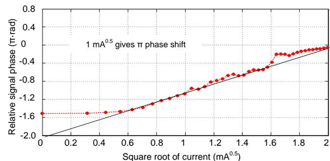
Fig. 20. Measured relative signal phase change.
