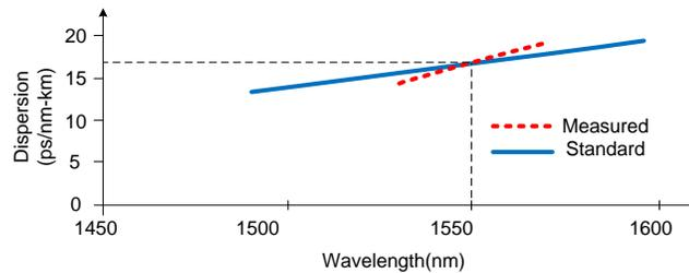
Fig. 11. Comparison of the measured dispersion of a 2-meter SMF and its standard dispersion value.
