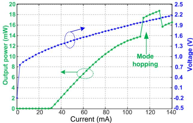
Fig. 14. Measured LIV curve of a SG-DBR laser.
