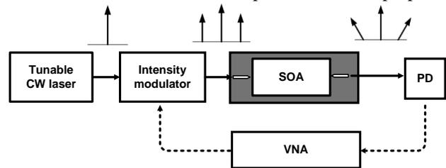
Fig. 10. SOA dispersion measurement setup
