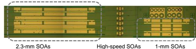
Fig. 3. Photo of the fabricated SOAs with different lengths. (left) 2.3-mm SOAs consisting of three cascaded SOAs with a length of 766  $\mu m$ ; (middle) high-speed SOAs with a length of 50, 100 and 150  $\mu m$ ; (right) 1-mm SOAs consisting of three identical SOAs with a length of 333 $\mu m$ .
