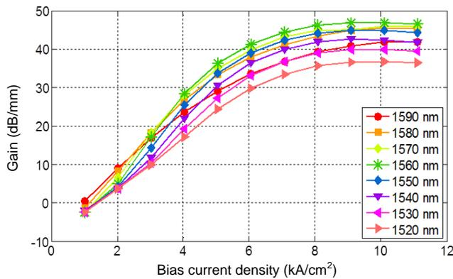
Fig. 7. Measured linear gain of a 1-mm SOA;
