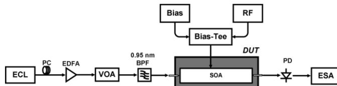
Fig. 4. SOA lifetime measurement setup
