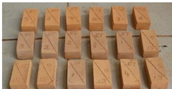
Image 1. Red mud bricks as derived from bauxite waste. (Agyei-Tuffour, Annan, Buabeng, et. al. )
