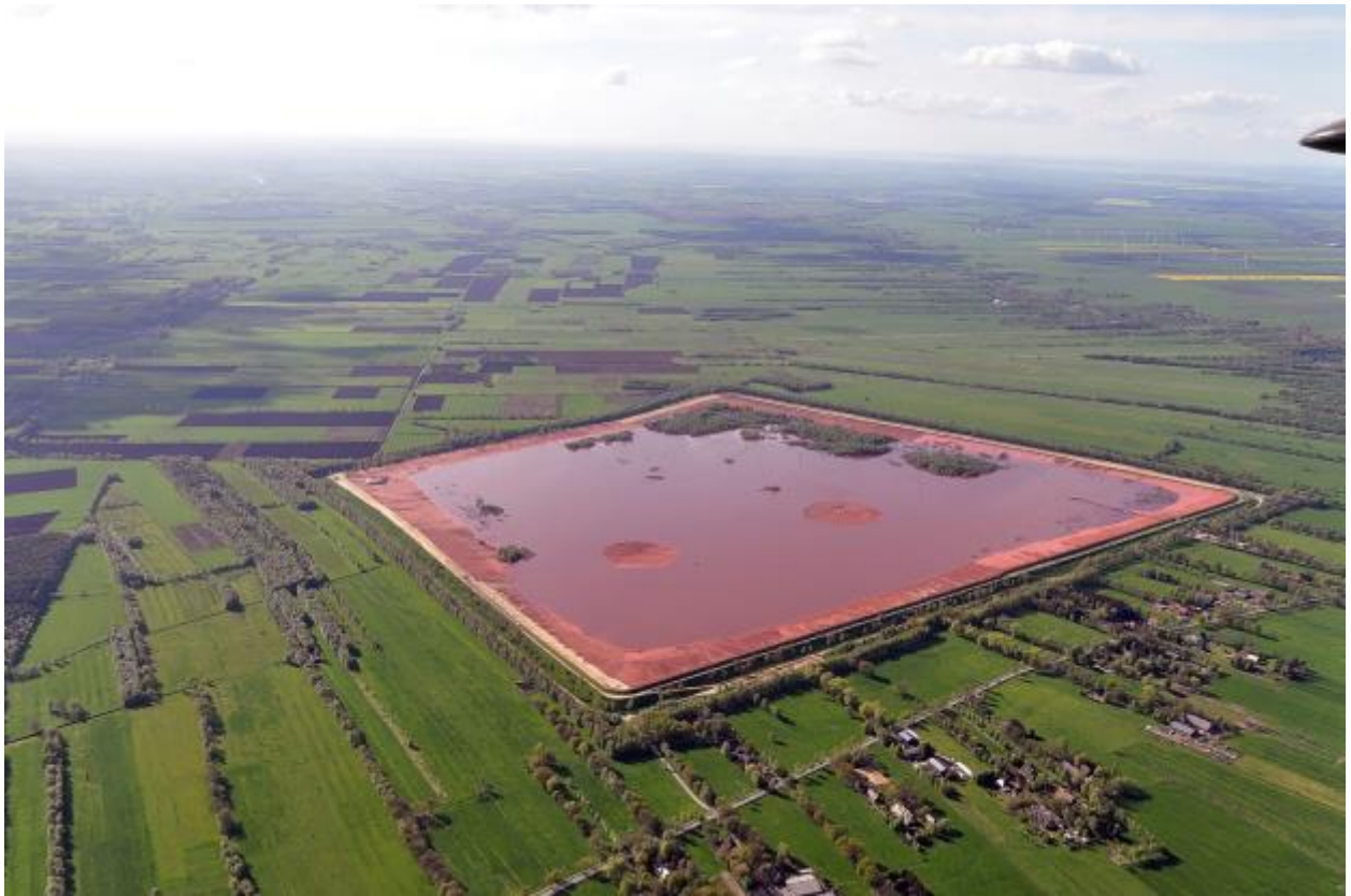
Image 1: Open-air storage of bauxite waste sludge.
