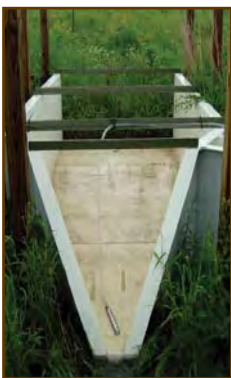
A flume measuring outflow from a 100% prairie field. Note the absence of sediment.
