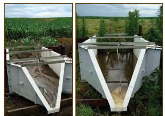
These flumes measure runoff from the STRIPS watersheds. Note the amount of sediment displaced from a 100% no-till crop field (left) compared to a field enhanced with 10% prairie (right).
