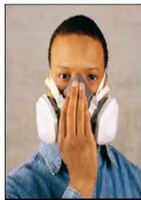
Place the palm of your hand over the exhalation valve cover and exhale gently. The facepiece should bulge slightly. If air leaks between the face and the facesal, reposition it and adjust the straps for a more secure seal.
