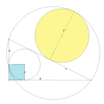
Using equivalent area formulae,  $\frac{ab}{2} = \frac{r(a+b+c)}{2}$ , this is easily seen to be  $y = \frac{a+b+c}{4}$ .
