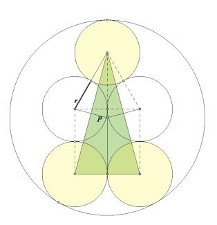
It is easier to work with radii geometrically. Let *O* be the center of one of the arcs. *O*, the center of either small circle, and its farther point of contact with the arc are collinear.
