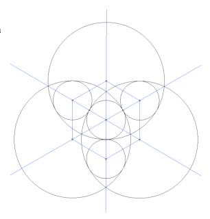
The median of an equilateral triangle of side s is  $\frac{s\sqrt{3}}{2}$ . The incenter trisects this segment; therefore, the inradius is  $\frac{s\sqrt{3}}{6}$ . Draw a tangent to the large circle where one of the small circles touches it. Its distance to the parallel chord is clearly  $s\sqrt{3}$ , so the large circle has radius  $s\sqrt{3} - \frac{s\sqrt{3}}{6} = \frac{5s\sqrt{3}}{6}$ , which is five times the radius of the smaller circles.
