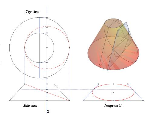
bases are the diameters parallel to  $\Sigma$ , and the segments joining their endpoints form an isosceles trapezium circumscribing the image of the ellipse. The image is also an ellipse, and one of its axes (in the orthographic drawing, the major axis) is the minor axis of the pre-image. The claim in the problem follows from applying the lemma to the whole image.
