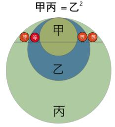
Given this figure with red circles of equal diameter, prove that the product of the diameters of the large and small green circles is the square of the diameter of the blue circle.
