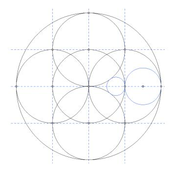
Say that the radii of the large black, blue, and red circles are r. The radii of the smaller black circles are  $\frac{r}{2}$ ; the radius of the image of the blue circle is  $\frac{r^2}{|(2r)^2-r^2|} \cdot r = \frac{r}{3}; \text{ and the radius}$  of the image of red circle is  $\frac{r^2}{|(4r)^2-r^2|} \cdot r = \frac{r}{15}.$
