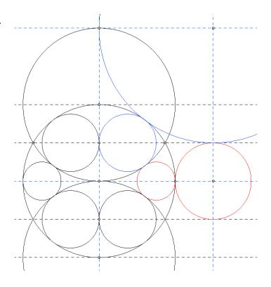
Draw (A)B with radius r;  $b \perp AB$  at B;  $c \perp AC$  at C;  $d \perp AC$  at D, the midpiont of AC;  $e \perp AB$  at E, the midpiont of BD; (B)E meeting AB produced in F; (A)F meeting e in G; and finally (G), which by construction touches (A)B, b, and d. (G) has radius  $\frac{3}{4}r$ .
