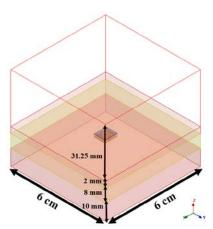
Fig. 3. Simulation set-up used to design the proposed antenna, which is placed directly under the 2mm skin layer.
