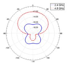
Fig. 4. Realized gain (dB) radiation pattern of the proposed implantable antenna vs. polar angle (coordinate system defined in Fig. 2).
