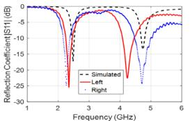
Fig. 8. Simulated vs. measured reflection coefficient  $(|S_{11}|)$  of the implantable antenna inside of the PMHS thigh.
