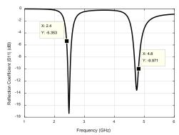
Fig. 5. Simulated antenna reflection coefficient vs. frequency.
