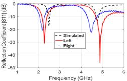
Fig. 9. Simulated vs. measured reflection coefficient  $(|S_{11}|)$  of the implantable antenna inside of the PMHS hip.
