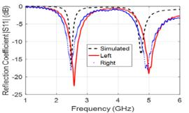
Fig. 10. Simulated vs. measured reflection coefficient  $(|S_{11}|)$  of the implantable antenna inside of the PMHS abdomen.
