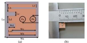
Fig. 1. Proposed 2.4/4.8 GHz implantable antenna: (a) model with dimensions shown in Table II, and (b) fabricated prototype.
