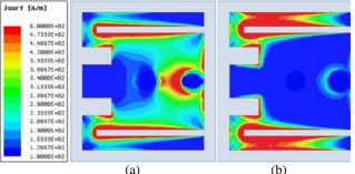
Fig. 2. Simulated current densities of the implantable antenna at (a) 2.4 GHz, and (b) 4.8 GHz.
