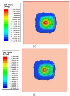
Fig. 6.  $SAR_{1g}$  simulations at: a) 2.4 GHz (input power = 4.75 mW), and b) 4.8 GHz (input power = 2.80 mW).
