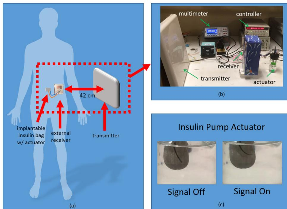
Visual Summary. (a) Illustration of application: transmitter delivers power wirelessly to on-body rectenna, which activates insulin pump, (b) test bench experiment, (c) wirelessly activated insulin pump arm
