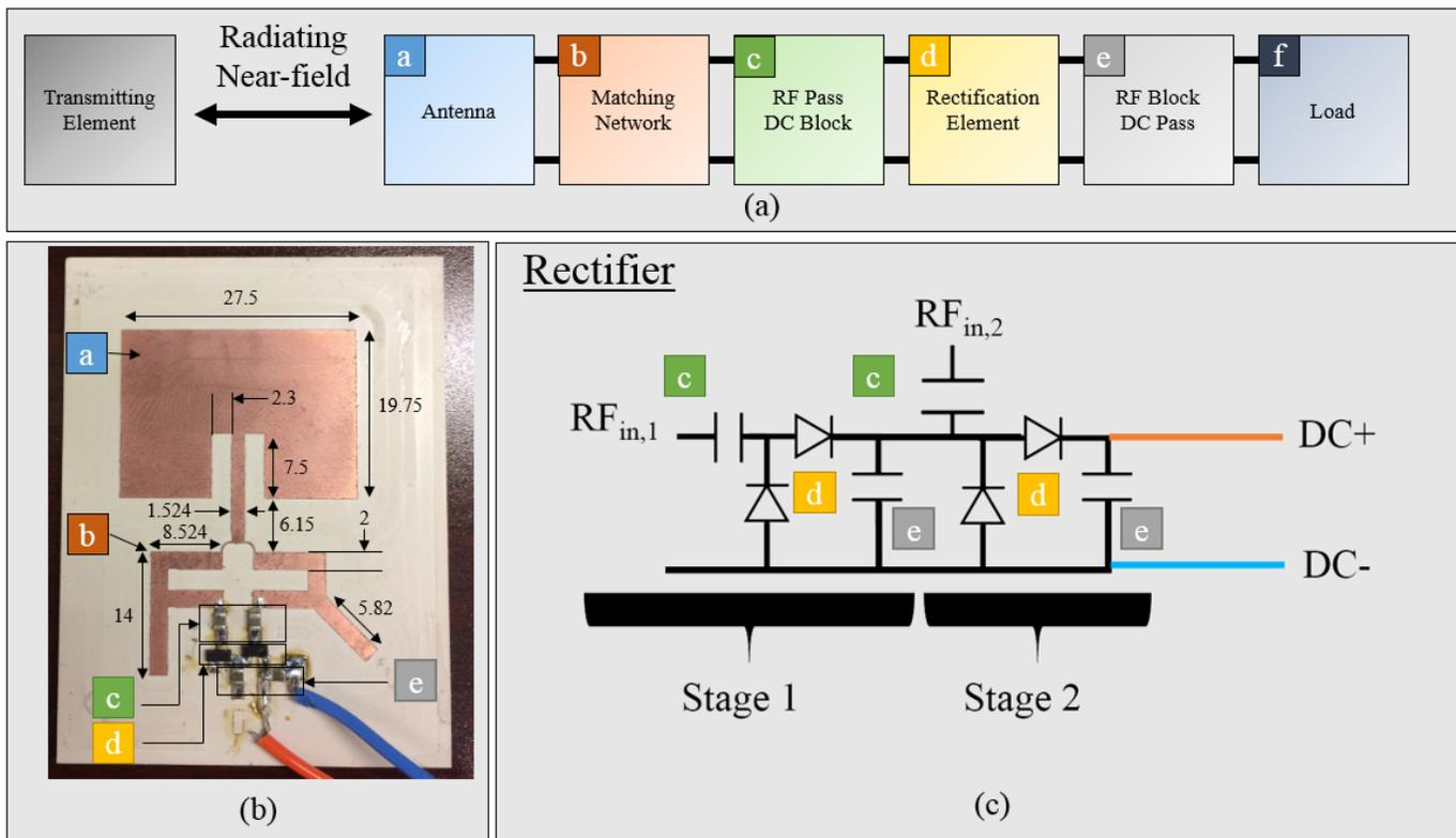
Fig. 1. (a) RF chain of the rectenna system, (b) fabricated rectenna circuit showing dimensions (all dimension are in mm), (c) circuit schematic of the equivalent voltage quadrupling rectifier
