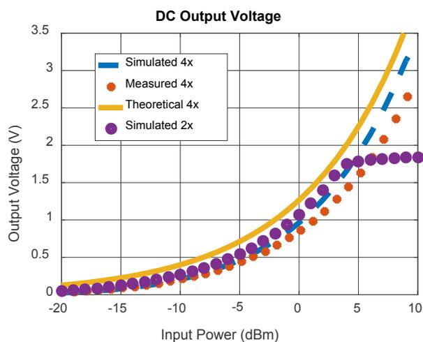
Fig. 2. Simulated, measured, and theoretical output voltage from voltage quadrupler, and simulated output from a voltage doubler
