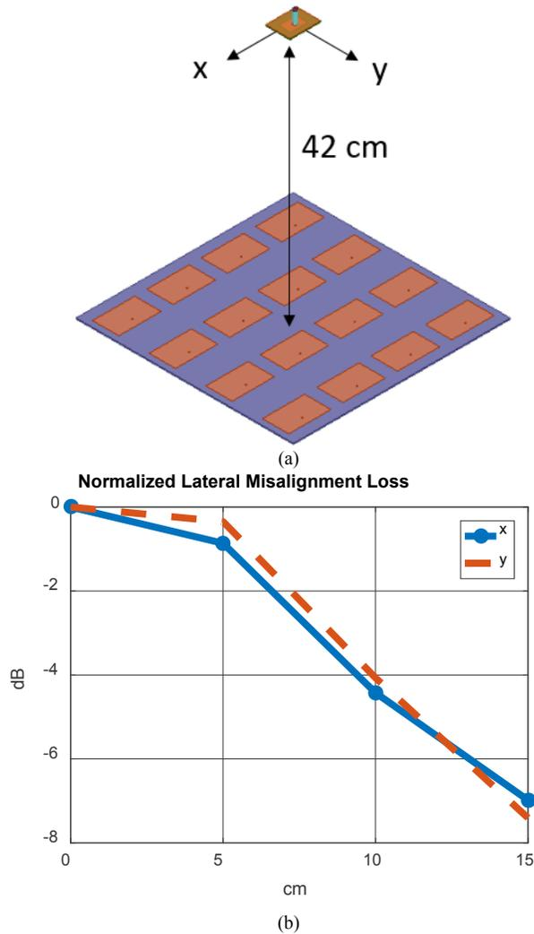
Fig. 4. (a) Illustration of the transmitting and receiving antenna in the lateral misalignment test, and (b) lateral misalignment loss as a function of offset distance when the vertical separation is fixed to 42 cm
