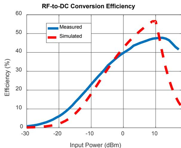
Fig. 3. RF-to-DC conversion efficiency of the voltage quadrupling rectifier
