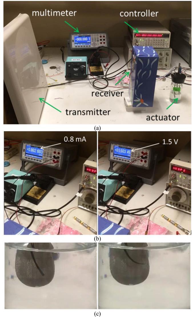
Fig. 5. (a) Radiating near-field rectenna setup, (b) measured voltage and current across 1.8 kΩ load, (c) actuated medical pump
