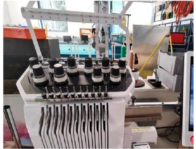
FIGURE 1. Specialist digital embroidery machine at Loughborough University for embroidering conductive threads. The designs can be converted into a picture and then fabricated automatically. It is important to be able to control the machine tensions as the threads are designed for their conductivities not their physical properties. The machine can also control the stitch spacing and direction.
