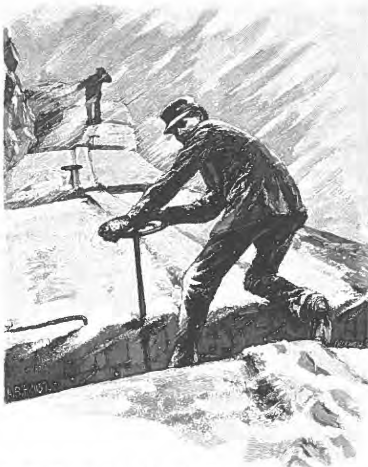
The hand brake system made the job of brakeman particularly perilous. (Reprinted from T. C. Clarke et al., The American Railway , New York, 1889.)
