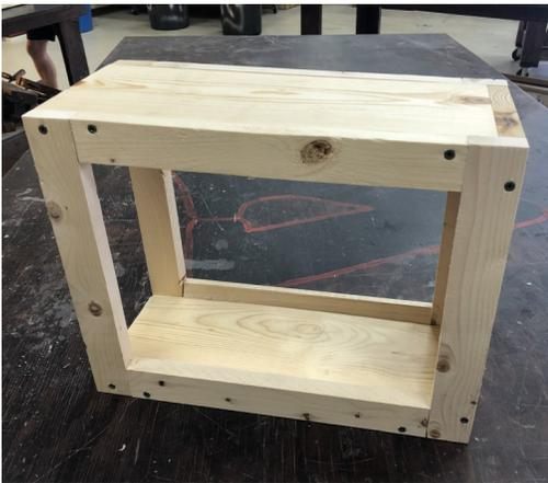
6. Again, to prevent splitting the wood, predrill two holes on each of the four boards framing the back of the box. Apply wood glue and screw in each of the four boards to create the back frame. (Photos 4 and 5)
