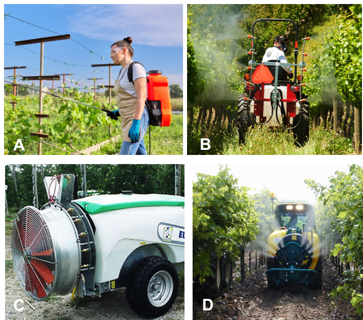
Figure 1. Examples of sprayers used in the vineyard or orchard. A) Backpack sprayer. B) Sprayer with vertical boom. C) Air-assisted sprayer. D) Tree-point-hitch air-shear sprayer. Photo C by Erdal Ozkan, The Ohio State University.
