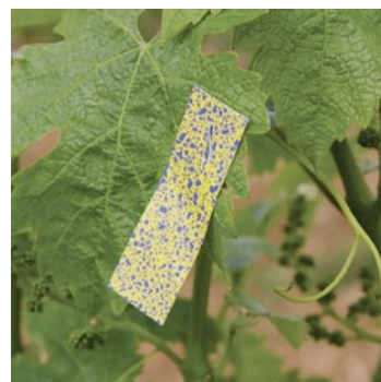
Figure 2. Water-sensitive papers are used to determine the location and uniformity of pesticide applications.
