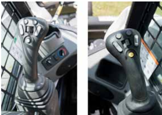
Figure 4.7 Joystick controls reduce operator fatigue. The joystick can be rotated to many positions and has finger-tip button controls to move the skid steer, raise/lower lift arms, tip the bucket, and operate hydraulically powered accessories. Credit: J. Mathison.
