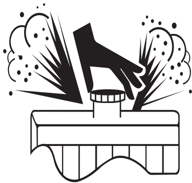
Figure 2.36 Never remove a radiator cap from a hot engine. Steam and hot water from the radiator can scald your skin. Credit: Association of Equipment Manufacturers.
