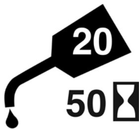
Figure 2.21 Universal symbols provide operating information. The oil can symbol may be used to indicate frequency of oil changes and the SAE number of oil to use. This picture represents an SAW 20 oil changed at 50 hours. Credit: J. Mathison.
