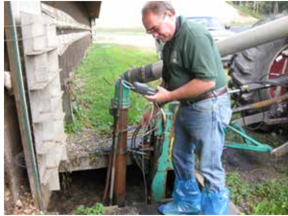
Figure 8.15 Always remain outside the manure storage facility when taking initial gas measurements. Credit: PSU Ag Safety.
