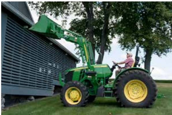
Figure 4.23 Extending the front-end loader with the bucket or fork attachment moves bulky loads easily, but also raises the tractor's center of gravity. This can allow the tractor to tip sideways more easily. Use the operator's manual to determine safe loading capacity. Credit: J. Mathison.
