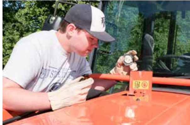
Figure 2.35 Before driving the tractor to the field, check for the possibility of an empty fuel tank. If you run out of fuel during a workday, it causes avoidable downtime. Credit: J. Mathison.
