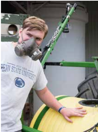
Figure 5.21 The chemical cartridge respirator mask has a replaceable filter to trap dust, chaff, and larger particles. These respirators will protect against toxic dust and light chemical vapors. They do not supply oxygen. Credit: J. Mathison.
