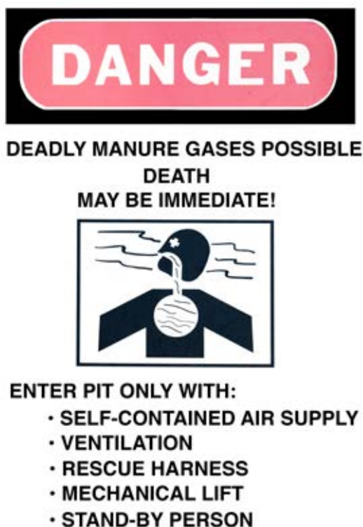
Figure 8.14 A danger sign posted near a manure storage structure provides a clear warning that immediate death is possible from manure gases. Credit: J. Mathison.
