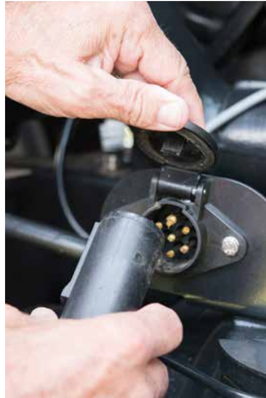
Figure 3.34 Align the pins of the electrical connection before attaching. Do not force the connector if the pins are not aligned. Threaded connectors do not pull loose; unscrew them first. Credit: J. Mathison.
