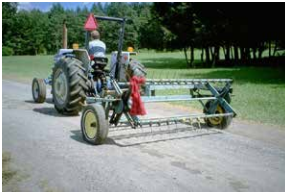
Figure 3.8 Implements can be wider than the tractor in transport or road position. Passing through farm gates or using public roadways can create a hazardous situation. Credit: J. Mathison
