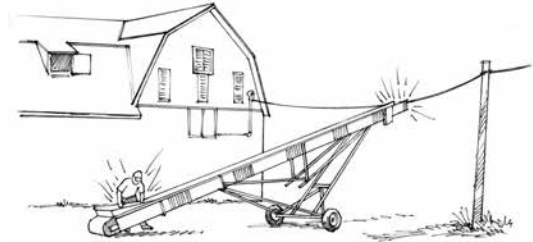
Figure 4.28 Lower an auger or elevator for transport to reduce risk of contacting overhead power lines. Credit: J. Mathison.
