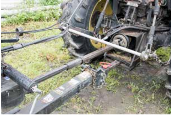
Figure 3.23 PTO shielding can be missing, bent, or inadequate. Notice that the guard for the implement drive shaft is missing, the tractor master shield is bent, and the tractor master shield does not provide protection for the driveshaft U joint. Youth should not operate PTO-powered machines that are not properly guarded. Credit: J. Mathison.
