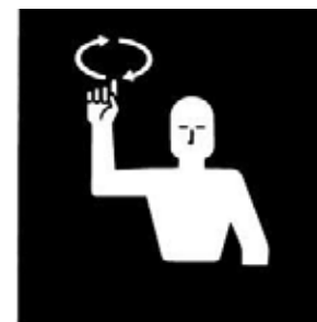
Figure 1.40 Raise the equipment. Make circular motion with either hand at head level. Example: Use this signal to have operator raise high lift or machine header.
