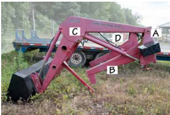
Figure 4.21 Front-end loaders may be parked and then will need to be mounted to the tractor you will operate. Components include: A. The tower columns, which are hooked to the tractor's mid-frame and often serve as the support legs. Some smaller units may have a light-duty rod that is inserted as the support leg. B. Bar and saddle, which hooks to the tractor's front frame. C. The lift arms and frame. D. The hydraulic control system. Study the components before attempting to connect to the tractor. Tighten all connections securely. Credit: J. Mathison.
