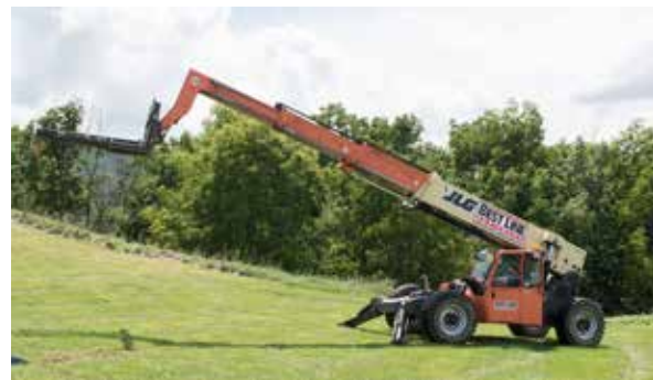
Figure 4.16 Telehandlers can handle large and weighty agricultural materials. Credit: J. Mathison.
