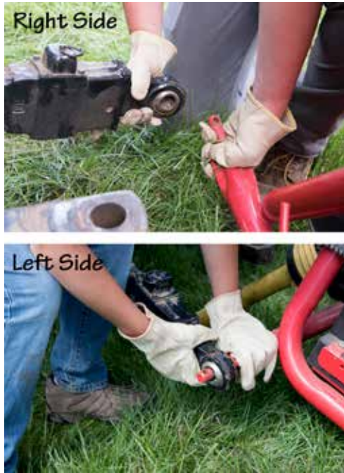
Figure 3.9 On both the left and right sides of the implement, insert the draft arm attachment pin of the tractor into the pin holes of the implement's lower hitch assembly. Secure the hitch with the proper size hitch pins and security clips. Credit: J. Mathison.
