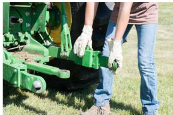
Figure 3.13 If the 3-point hitch is equipped with an extension to the lower draft arm, release the lock and pull or extend the draft arm extension to the rear before nearing the implement to be attached. Credit: J. Mathison.
