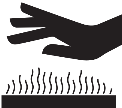
Figure 3.26 Hydraulic hoses and fittings can become hot during use. Place your hand near them to check for heating. Do not just grab them! Credit: Association of Equipment Manufacturers.
