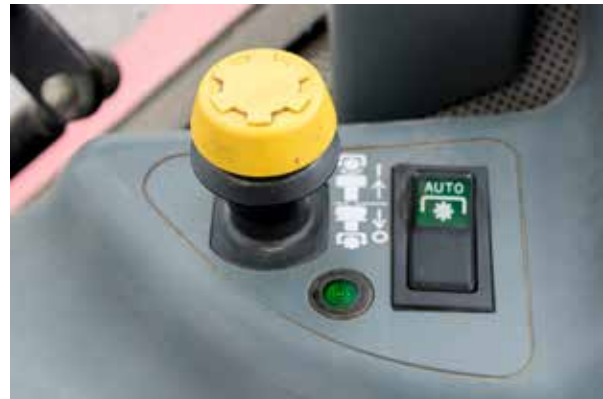
Figure 2.14 A hand-operated PTO control. Credit: J. Mathison.
