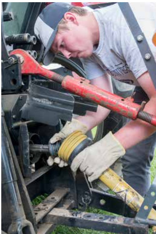
Figure 3.12 To attach the PTO shaft, you will be operating in a crowded space. Be sure the tractor is securely parked and the engine is shut off. Credit: J. Mathison.
