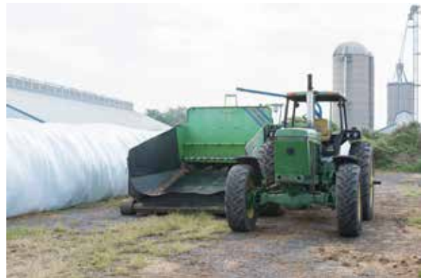
Figure 4.31 Silage bagging equipment is driven by the PTO of the bagging tractor. A second tractor or dump truck and unloading equipment is operated in close proximity to the tractor and bagging equipment and must be moved slowly forward as the bag is filled. The bag being filled is directly behind the tractor. Credit: J. Mathison.
