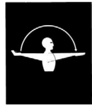
Figure 1.33 Move out—take off. Face the desired direction of movement; hold the arm extended to the rear; then swing the arm overhead and forward in the direction of desired movement until the arm is horizontal with palm down. Example: You have hitched the machine for the operator and connected the PTO. After you are out from between the tractor and the implement, signal the operator to move out for field work.
