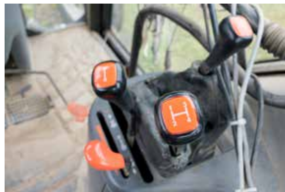
Figure 2.8 Ground motion controls include transmission controls, park-lock, and gear-shift levers. Credit: J. Mathison.
