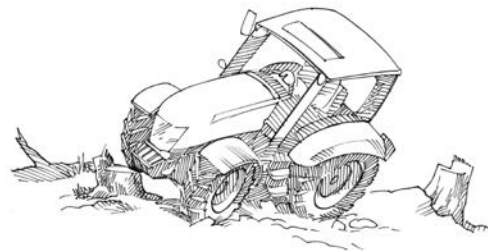
Figure 2.69 Avoid obstacles as you operate the tractor. Some tractor operators will check the field before beginning the operation. Stumps, rocks, animal dens, etc., can upset a tractor. Credit: J. Mathison.
