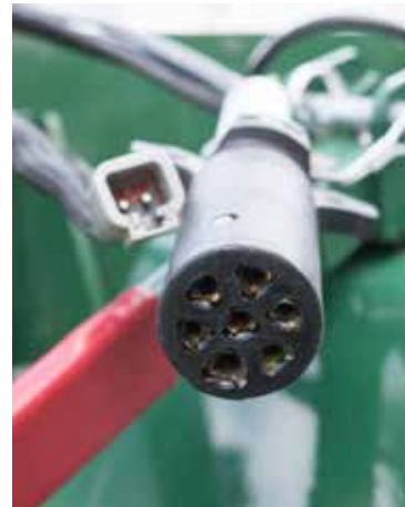
Figure 3.32 Some connected implements need electrical power. Connectors may have prongs with screw-in couplings to keep them from vibrating loose. Other connectors may be plug types that are simply pushed together (shown here). Recognize the difference to avoid damage when connecting or disconnecting them. Credit: J. Mathison.
