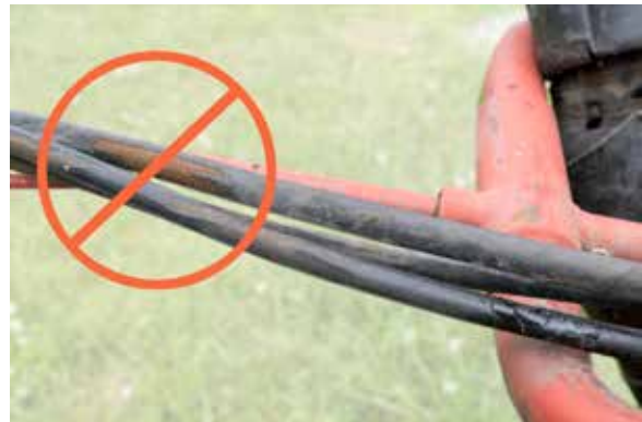
Figure 3.27 Hydraulic hoses may be reinforced, but damage to the outer covering, plus pinholes from high pressure, can cause serious injury (e.g., amputation) and machinery downtime. Credit: J. Mathison.
