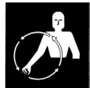
Figure 1.37 Start the engine. Move arm in circular motion at waist level to simulate cranking engine. Example: You need to signal the operator to start the tractor engine.
