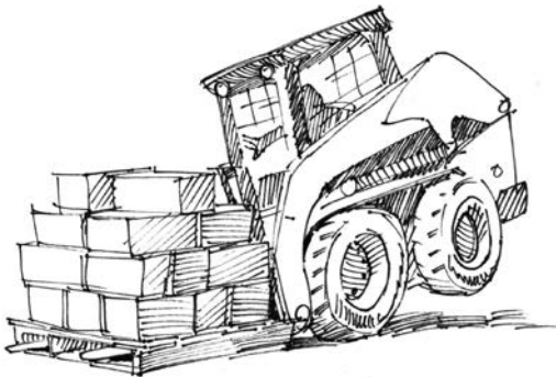
Figure 4.3 Skid steer loaders can tip forward if overloaded. This is an important reason to wear your seat belt and to understand the skid loader's load limitations. Credit: J. Mathison.
