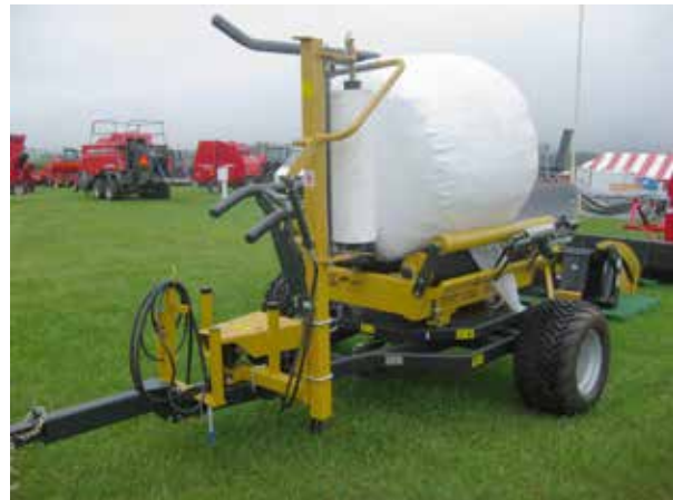
Figure 4.33 The bale wrapper uses hydraulic components to rotate the bale in two directions to wrap the plastic film snugly. Once covered, a shear arm cuts the plastic, the bale is dropped to the ground, and another bale is lifted into place for wrapping. Because this is done from the tractor seat, the operator is physically removed from machine hazards. Keep children and bystanders away from the wrapping operation. Credit: J. Mathison.
