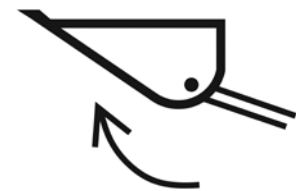
Figure 2.31 This symbol indicates that the resulting operation will tilt the high-lift bucket to the rear. Credit: J. Mathison.
