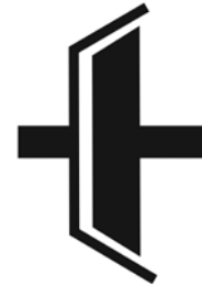
Figure 2.29 This symbol shows whether the clutch is engaged or disengaged. Credit: J. Mathison.
