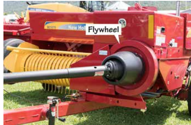
Figure 1.7 The flywheel on a small square baler is an example of a freewheeling part. The flywheel keeps the baler running smoothly if a large amount of hay is suddenly taken into the bale chamber. The PTO is properly guarded. Credit: J. Mathison.
