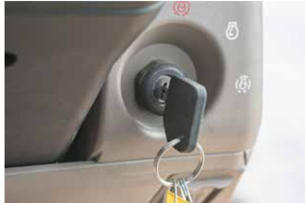
Figure 2.45 Turn the ignition key to the start position. Do not hold the key there for extended periods of time. This can burn up the starter motor or drain the battery of its charge. Credit: J. Mathison.
