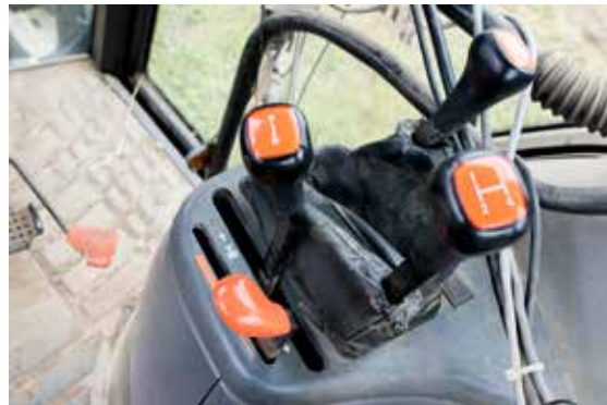
Figure 2.47 Remember that orange-colored control levers indicate ground motion controls. Study the gear shift pattern on the tractor you are operating. Use a lower gear to start the tractor moving. Use a higher gear for operation. Higher gear use with heavy loads may stall the engine or cause rearward overturns. If the shift pattern is difficult to locate, ask someone who is familiar with the tractor to show you the shift pattern. Credit: J. Mathison.
