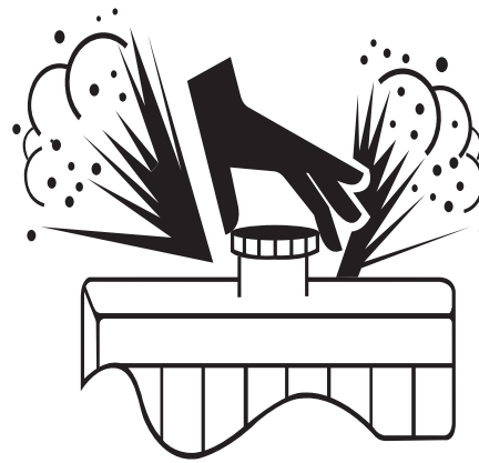
Figure 1.29 Caution: Hot fluid under pressure. Credit: Association of Equipment Manufacturers.
