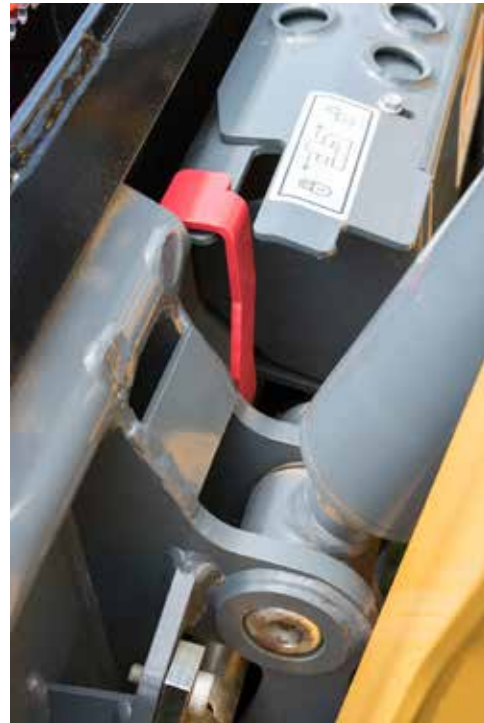
Figure 4.9 If the skid steer loader mounting plate does not have latch handles to lock the attachment, look for the hydraulically operated pins that provide the locking mechanism, and for the hydraulic control that activates the lock pin. Credit: J. Mathison.
