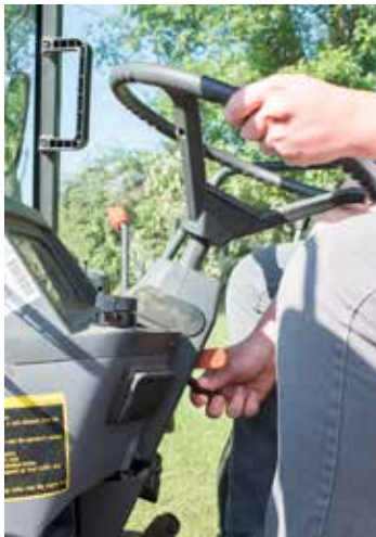
Figure 2.43 The steering wheel should be adjusted as soon as you are seated. In the correct position, your arms are bent at a 90-degree angle as you hold the steering wheel. Credit: J. Mathison.
