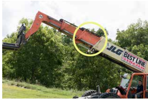
Figure 4.17 As the boom is extended, a letter or number marking (circled) is revealed with references in the operator's cab to give restrictions on how much weight can be lifted safely. A boom angle indicator is included. Credit: J. Mathison.
