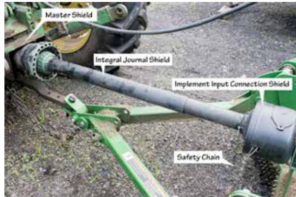
Figure 3.22 The major guards of a PTO system. The implement input connection (IIC) shield protects the operator from the IIC, including the implement input stub and the connection to the implement input driveline (IID). The safety chain keeps the integral journal shield from spinning and shows that the shield is not stuck to the IID. The safety chain should be replaced immediately if damaged or broken. The master shield protects the operator from the PTO stub and the connection of the IID to the PTO stub. The integral journal shield completely encloses the IID, may be made of plastic or metal, and is mounted on bearings to allow it to spin freely from the IID. The integral journal shield should always be checked before operation for free movement. Credit: J. Mathison.
