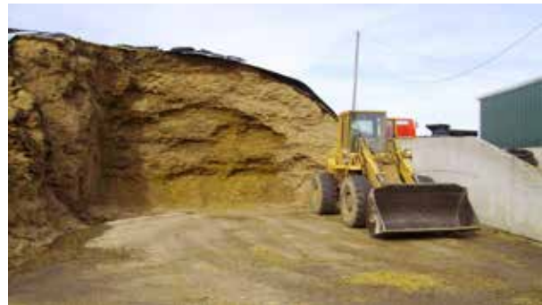
Figure 4.29 This loader may be large enough for most jobs, but it cannot reach the top of this silage pile to evenly remove the silage each day. Collapse of the silage face can entrap a worker when the silage face caves in from being undercut. Credit: J. Mathison.
