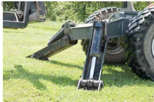
Figure 4.19 If the telehandler is equipped with outriggers, use them to stabilize the machine during stationary use. Credit: J. Mathison.
