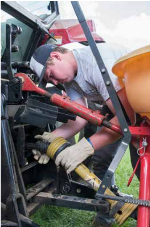
Figure 3.20 This is what the task of connecting a PTO shaft looks like. You must lift a heavy object at an awkward angle while squeezing in the lock mechanism detent pin. Watch someone else connect a PTO several times before doing this job. Credit: J. Mathison.
