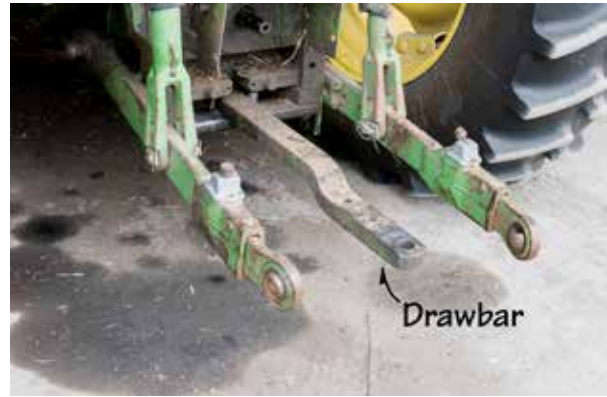
Figure 2.60 Only hitch to the drawbar. Credit: J. Mathison.
