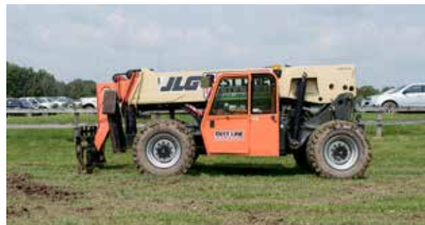
Figure 4.20 When finished with work, park on level ground with the boom retracted and lowered. Set the park brake. Remove the keys so that an untrained person cannot move the machine. Credit: J. Mathison.
