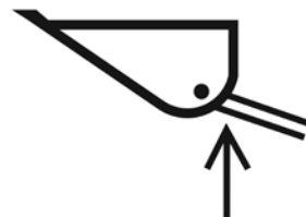
Figure 2.30 This symbol indicates that the resulting operation will raise the high-lift bucket. This is a positioning and adjusting control symbol. Credit: J. Mathison.
