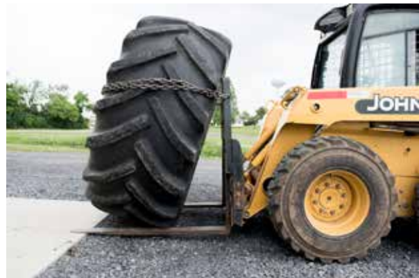
Figure 4.5 Return lift arm and skid steer attachments to ground level when stopping the machine. This allows a safe exit of the cab because you can't accidentally bump the control levers and lower the components on yourself or others. Credit: J. Mathison.
