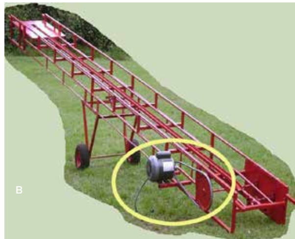
Figure 4.27a and b (a) An elevator that can be used for a variety of agricultural products. (b) An elevator for moving hay or straw. Note the turning parts (motor pulley, belt, and drive pulley), as well as the open frame structure. Homemade elevators may be made with solid wooden sides and bottom. Because of the unguarded pulleys and belt, this is an unsafe drive mechanism. Credit: (a) PSU Ag Safety (b) J. Mathison.
