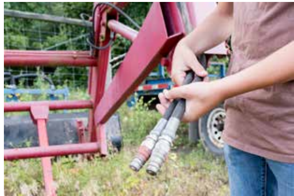
Figure 3.30 The male half of the coupler is part of the cylinder or hydraulic device system. Be sure to wipe dirt and grime from the hose end fitting. Credit: J. Mathison.
