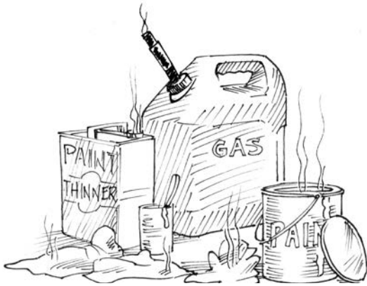
Figure 5.35 Vapors are produced by cleaning solvents, gas, and paints. Vapors that pass off into the atmosphere are termed “volatile.” Credit: J. Mathison.
