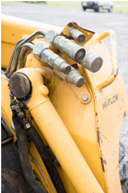
Figure 4.11 Hydraulic hoses are attached to the skid steer at conveniently located quick connection points. Credit: J. Mathison.
