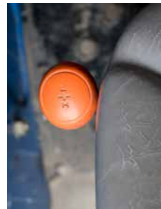
Figure 2.49c A high-low range shift lever found near the stick shift provides a faster or slower speed for a particular gear. These symbols may be missing or worn, causing the operator to have to ask for assistance or to locate the gear pattern themselves. Credit: J. Mathison.
