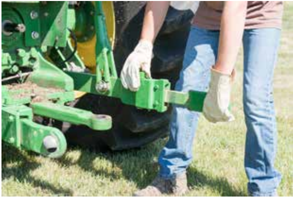
Figure 3.14 The telescopic extension to the draft arm is fully extended. In some cases, this must be done to align with the lower lift points of the 3-point hitch implement. Be sure the extension is pushed back into the draft arm until locked into place when you are finished attaching the implement. Credit: J. Mathison.
