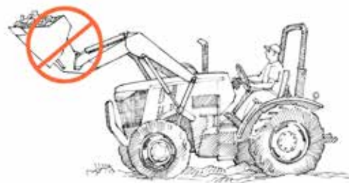
Figure 4.22 When operating the front-end loader, keep the loaded or empty bucket as low to the ground as possible while in transport. Sideways rollovers can result if you travel with the bucket in the up position. Credit: J. Mathison.
