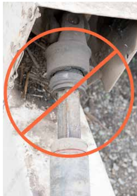
Figure 2.3 Tractors provide remote power to machinery. This turning shaft, the PTO, must be guarded to prevent entanglement hazards. The PTO shown here is unguarded and very dangerous. Credit: J. Mathison.
