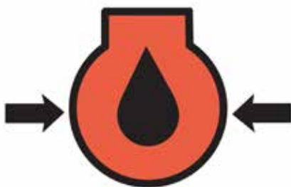
Figure 2.26 The engine oil pressure symbol draws your attention to malfunctions during operation. It glows red when pressure is insufficient. Credit: J. Mathison.
