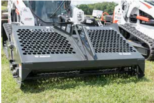
Figure 4.10 A hydraulically operated tiller attachment is shown. Credit: J. Mathison.
