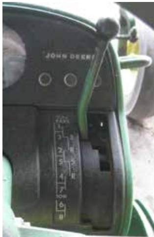
Figure 2.50 A synchronized shift transmission permits the operator to shift on the go within a range of "synchronized" gears. Credit: J. Mathison.
