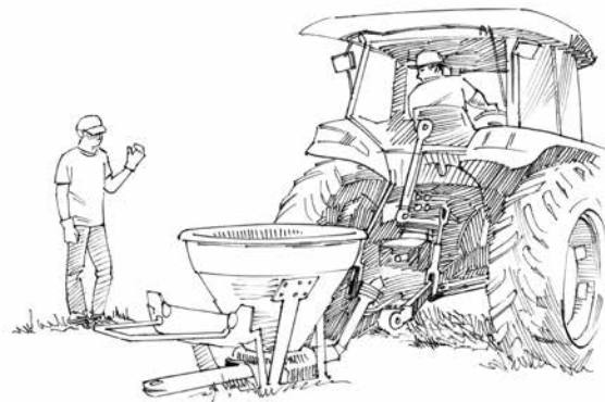
Figure 3.4 Never let another person stand between the tractor and the implement during hitching. Too fast of an approach or the operator's foot slipping from the clutch could lead to injury or fatality to the person standing nearby. Credit: J. Mathison.
