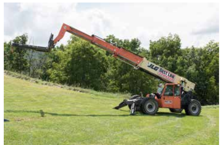
Figure 1.8 Hydraulic systems such as this telehandler often have stored energy. Credit: J. Mathison.
