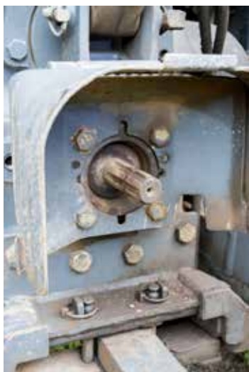
Figure 3.16 The 540-rpm PTO stub shaft has 6 splines or teeth and is 1 3/8 inch in diameter. Credit: J. Mathison.
