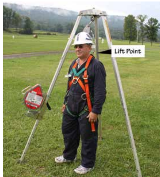
Figure 8.17 An appropriate body harness loops around both legs and the person's shoulders, and has a lifting point centered between the shoulders on the back so the person can be safely lifted by a winch. Credit: PSU Ag Safety.
