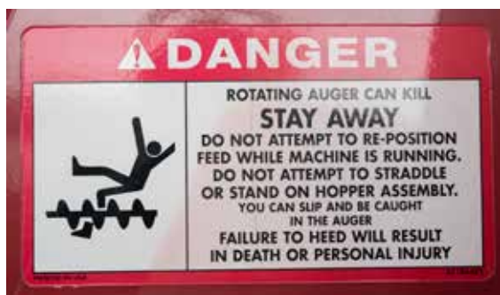
Figure 1.21 DANGER—These signs are RED and illustrate the most serious potential hazards. Credit: J. Mathison.
