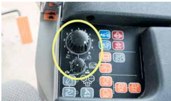
Figure 2.16 The two black knobs are lift controls for implements or attachments. Credit: J. Mathison.
