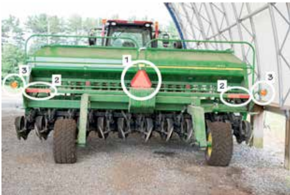
Figure 2.81 Can you identify the lighting and marking features used on this tractor and grain drill? No. 1 is _____. No. 2 are _____. No. 3 represents _____. Is the equipment safely marked for roadway travel? Credit: J. Mathison.
