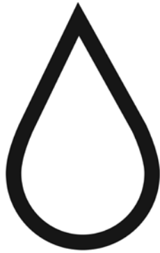
Figure 2.20 The symbol for oil should draw your attention to checking the oil or the oil fill area. You will see this symbol with engine lubricant and hydraulic systems. Credit: J. Mathison
