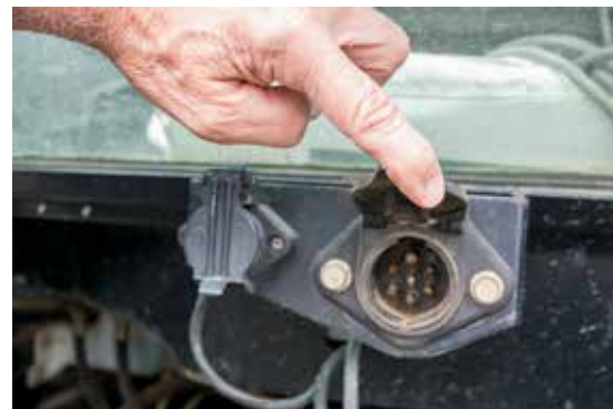
Figure 3.33 Electrical connectors are protected from dust, dirt, grease, and grime with dust caps. Keep these covers in good repair and in place to ensure that electrical connections can be made without delay. Credit: J. Mathison.
