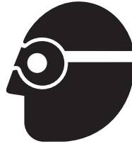
Figure 1.12 Goggles with impact-resistant lenses are recommended when you see this symbol. Goggles protect against splashes from all types of hazardous liquids. Credit: Association of Equipment Manufacturers.
