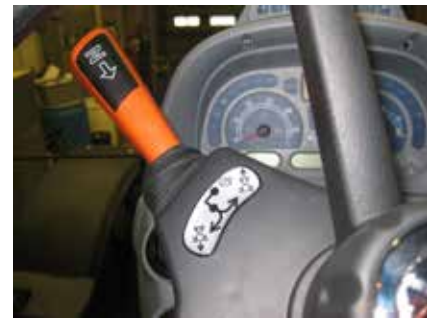
Figure 2.51 Look on the left side of the steering column. The shuttle shift lever, sometimes called the reverser, allows for ease of changing direction without using the clutch. This lever may serve as the positive park to be used with the parking brake. Some may have to be in a neutral position for the tractor to start. This may be the only time that the clutch pedal is used. Credit: J. Mathison.
