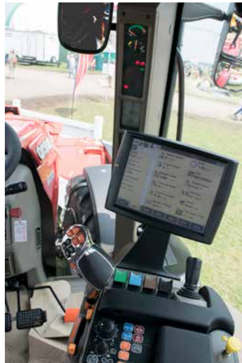
Figure 2.53 A contemporary tractor has sophisticated controls and monitoring systems. Use the operator's manual and ask your supervisor to explain the tractor's operation. Credit: J. Mathison.
