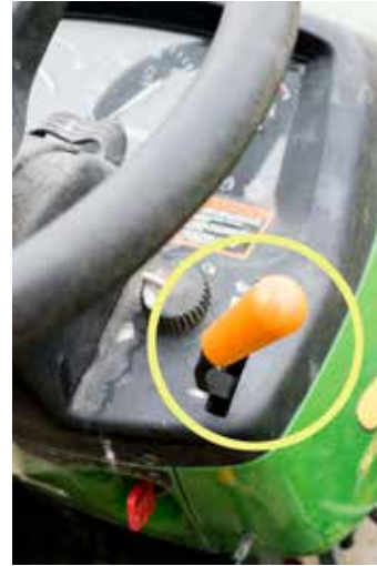
Figure 2.15 The ground speed control on the tractor is orange. Orange is the color code for ground motion controls. Credit: J. Mathison.
