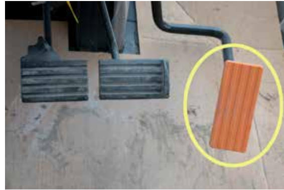
Figure 2.9a The foot throttle on this modern tractor is orange. Orange is the color code for ground motion controls. Credit: J. Mathison.
