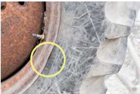
Figure 2.40 Damaged rims from careless use may cause damaged tire beads and flat tires. Credit: J. Mathison.
