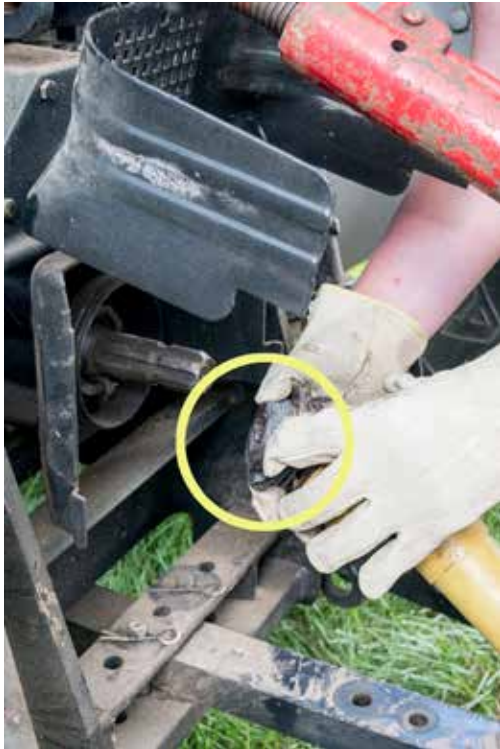
Figure 3.11 A firm grip will be needed to press in on the detent lock of the PTO shaft. This lock engages the groove in the stub shaft to secure the PTO driveline shaft to the stub shaft. There are also other forms of locking the PTO shaft. Credit: J. Mathison.
