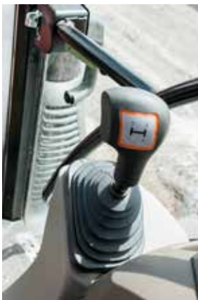
Figure 2.49a The typical “H” pattern gear shift choice. Credit: J. Mathison.
