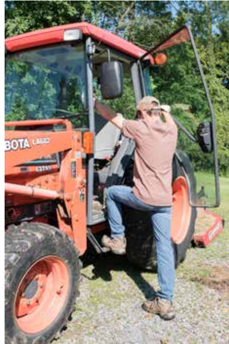
Figure 2.46 Mount a tractor safely by using the handholds and steps. Credit: J. Mathison.
