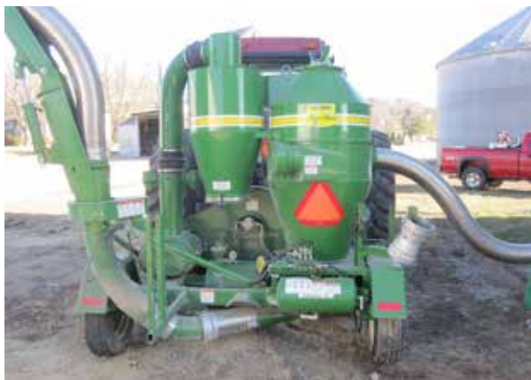
Figure 8.11 A grain vacuum moves large quantities of grain from storage to truck, or from truck to grain bin. Credit: J. Mathison.
