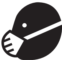
Figure 1.14 A NIOSH-approved dust mask is recommended when you see this symbol. An approved dust mask will always have two straps. Make sure that the mask fits snugly around your mouth and nose. Credit: Association of Equipment Manufacturers.
