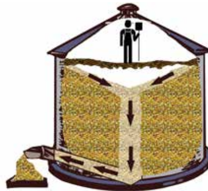
Figure 8.7 A “grain bridge” cannot support the weight of the worker. Credit: PSU Ag Safety.
