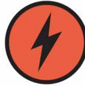
Figure 2.27 The ammeter or generator symbol draws your attention to malfunctions during operation. It glows red with insufficient charge rate. Credit: J. Mathison.
