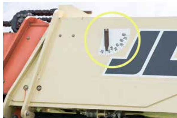
Figure 4.18 A close-up of the boom angle indicator, which is typically visible to the operator from the cab seat. A similar indicator is found on the instrument panel to show frame angle.
