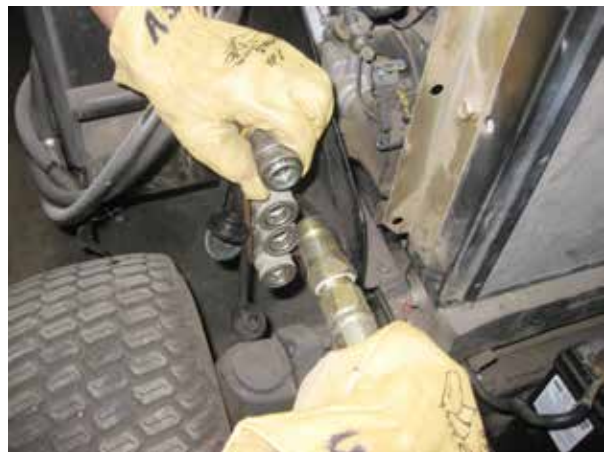
Figure 3.31 The lock ring of the female end of the coupling will secure the two fittings together. A firm grip is needed to insert the hydraulic hoses from the implement (male end) into the coupling on the tractor (female end). Credit: J. Mathison.
