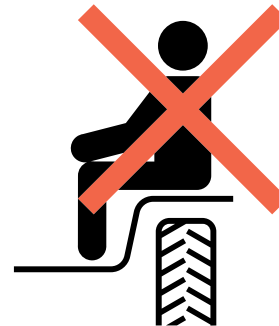
Figure 2.2 Tractor runovers have claimed many lives. Extra riders can slip from the tractor and be crushed before the operator can stop. Say no to your friends who want to hitch a ride. Credit: Association of Equipment Manufacturers.
