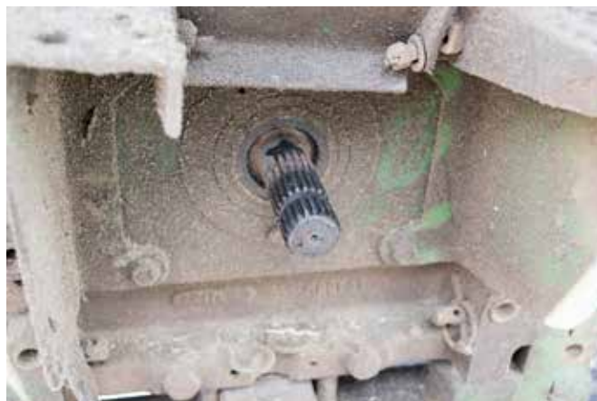
Figure 3.17 The 1,000-rpm PTO stub shaft has 20 splines or teeth with a 1 3/4-inch diameter. It could instead have 21 splines with a 1 3/8-inch diameter. Credit: J. Mathison.
