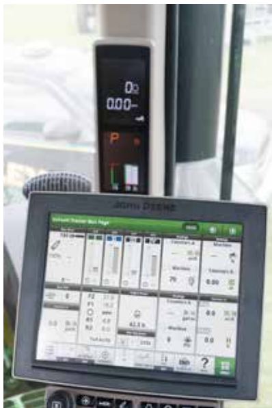
Figure 2.5 The modern tractor instrument panel may appear as complex as the cockpit controls of a jet airliner. The operator must know what each instrument or gauge is telling him/her about operating conditions. Credit: J. Mathison.
