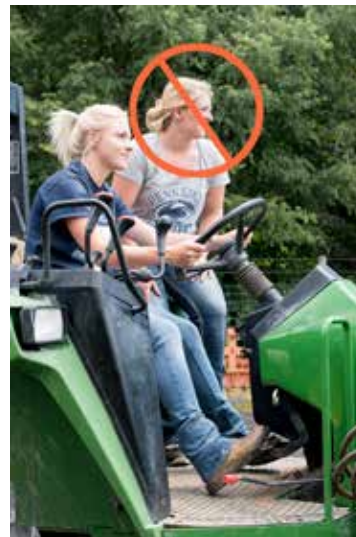
Figure 2.64 Tractors are designed for the operator only. No passengers allowed! Credit: J. Mathison.
