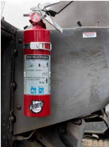
Figure 5.39 All tractors should have a dry chemical-type fire extinguisher on board. Today's high-priced tractors and equipment should be fire control ready. What class(es) of fire will the dry chemical extinguisher control? Credit: J. Mathison.
