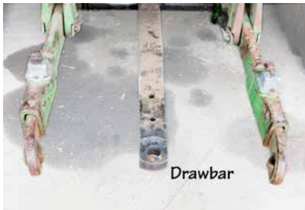
Figure 3.2 The tractor drawbar is the only safe place to connect a load. Do not hitch higher than the drawbar so all pulling forces stay below the tractor's center of gravity. For most operations the drawbar should be placed midway between the rear tires to maximize pulling power. Hillside operations may require a drawbar adjustment to one side to balance the pulling forces. Credit: J. Mathison.
