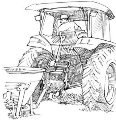
Figure 3.6 If the tongue of the implement is not adjusted for the height of the drawbar, the drawbar can push the implement to the rear, knock the jack stand over, or harm someone standing behind the implement. Taking a preliminary measurement of the drawbar height and the implement tongue before hitching makes aligning the two points much easier. A stable jack stand should be used. Credit: J. Mathison.
