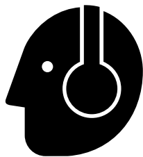
Figure 1.17 Hearing protection is recommended when you see this symbol. If you cannot hear a person standing 3 feet away talking in a normal voice, hearing protection is needed. Credit: Association of Equipment Manufacturers.
