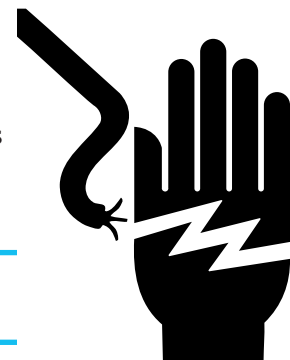
Figure 5.40 The pictorial symbol for electric shock hazard. Credit: Association of Equipment Manufacturers.
