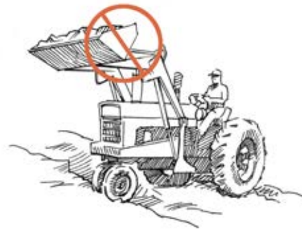
Figure 2.71 When operating a high-lift bucket with or without a load, keep the bucket as low to the ground as possible while in transit. Sideways overturns are possible if you travel with the bucket in the up position. Credit: J. Mathison.
