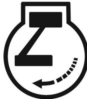
Figure 2.23 This symbol shows the engine speed (rotations per minute). Credit: J. Mathison.
