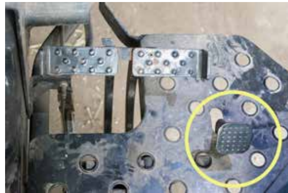
Figure 2.9b The foot throttle on this older tractor is black. Many older tractors won’t have the more modern color coding of controls. Credit: J. Mathison.
