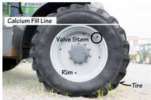
Figure 2.38 Tractor tire components include the tire, the rim or wheel, an inner tube with valve, and often a calcium solution filling about 80% of the inner tube. The calcium fill line is 80% if calcium or similar solution is used. Credit: J. Mathison.
