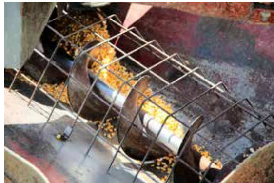
Figure 4.25 Augers are found in many places. Augers move grain and feedstuffs into bins and processors and carry these materials to feed carts, grinders-mixers, and feed bunks. The moving parts can pull a victim into the machine. Augers should be guarded as shown. Auger guards must be kept in safe condition. Credit: Central States Center for Agricultural Safety and Health.
