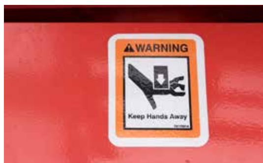
Figure 1.24 Potential crushing hazard to hands. Credit: J. Mathison.
