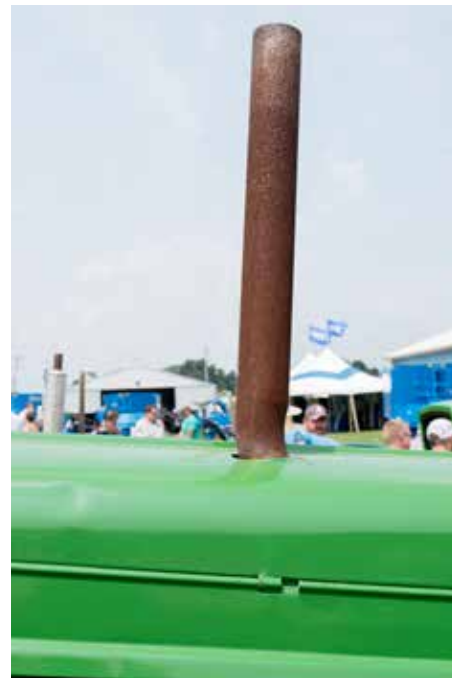
Figure 5.22 A straight pipe used for the exhaust or a worn-out muffler will increase noise levels coming from the engine. Muffler condition should be part of a safety audit. Credit: J. Mathison.
