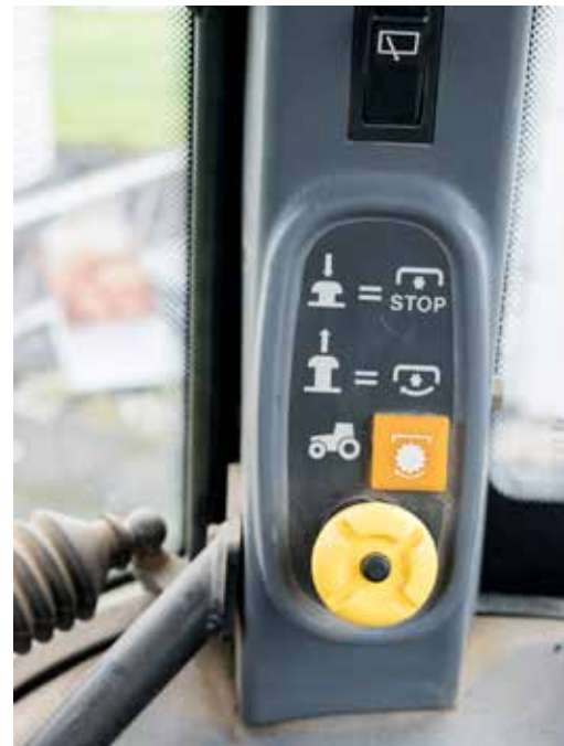
Figure 2.10 Yellow color-coded controls engage accessories. This is often done through the PTO control, an example of which is shown here. Credit: J. Mathison.
