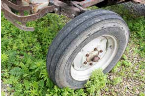
Figure 2.39 Worn tire treads and dry rot make for poor traction and risk downtime due to a blowout. Credit: J. Mathison.
