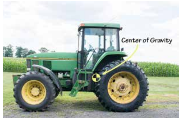
Figure 2.54 Expected position of a tractor's center of gravity. Credit: J. Mathison.
