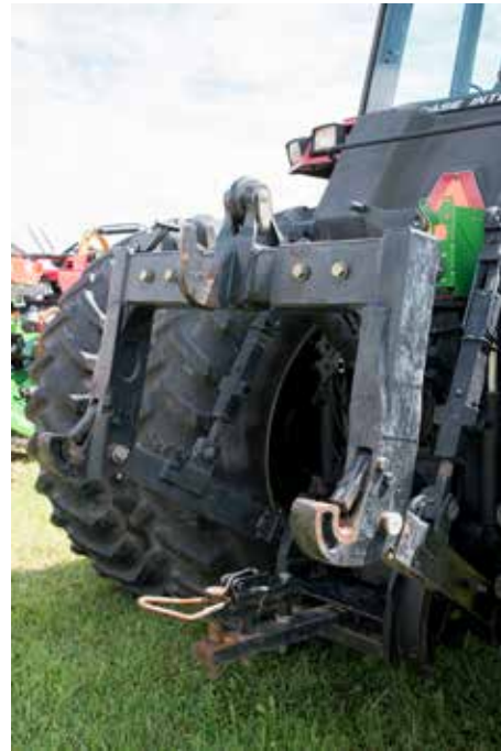
Figure 3.5 Heavy-duty quick-attach couplers are mounted onto the tractor's 3-point hitch and can safely handle large 3-point hitch implements without a person moving between the tractor and the implement. Refer to the operator's manual for additional instructions on their use or have a qualified operator demonstrate to you the correct procedure to use a quick-attach coupler. Credit: J. Mathison.
