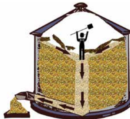
Figure 8.8 As the grain bridge gives way, the worker is pulled into the pocket and is engulfed. The grain auger may have been left running and the flowing grain pulls the victim under the grain. Credit: PSU Ag Safety.
