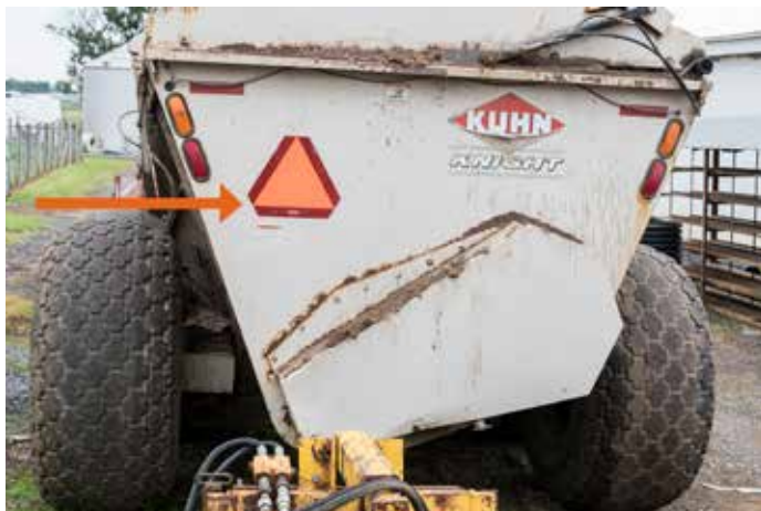
Figure 2.77 SMV emblems are required on vehicles designed to travel less than 25 mph while occupying public roadways. SMV emblems should be visible from no less than 1,000 feet to the rear of the tractor or towed implement. Therefore, mounting height may vary from 2 to 10 feet above the road surface. Replace faded, damaged SMV emblems. Credit: J. Mathison.
