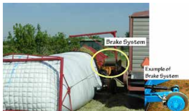
Figure 4.32 From the rear of the bagging equipment, the endgate and cable braking system are shown. A large industrial disc brake(s) (see inset) and a simple brake hand pump and brake pressure gauge control the rate of cable release. Silage bags may have convenient “stretch gauges” marked continually along the bag to ensure packing consistency. Tension may be preset with experience or manually controlled during fill. Tension on the cable is released from the endgate when the bag is filled, and the endgate can drop heavily to the ground. The close quarters between the bagging equipment and the wagon or truck being unloaded raise the potential for injury. Turning parts can snag loose clothes very quickly, and the tractor operator's visibility of someone in this space is reduced. Credit: PSU Ag Safety.
