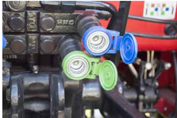
Figure 3.29 The female half of the hydraulic coupler is considered to be part of the tractor. Dust covers protect the quick release fitting, which includes the lock ring and ball lock mechanism. Credit: J. Mathison.
