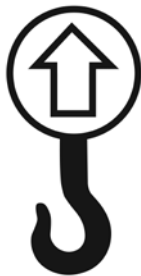
Figure 2.22 This symbol shows the only recommended lift point to attach a chain for moving a heavy weight. Damage or injury can occur if any other lift point is used. Credit: J. Mathison.
