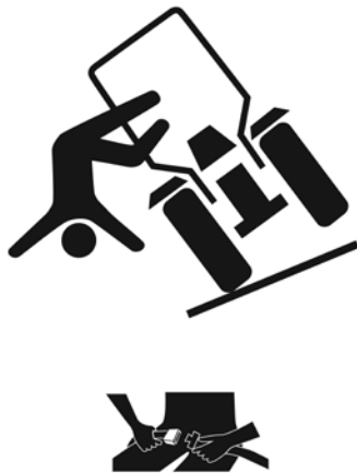
Figure 2.63 A rollover protection structure (ROPS) and a seat belt can protect you in the event of an overturn. If you are in the cab of a ROPS-equipped tractor, fasten the seat belt. Credit: J. Mathison.
