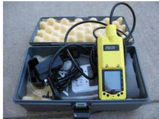
Figure 8.16 Hand-held, portable multi-gas monitors measure most of the manure gases and oxygen levels. Credit: PSU Ag Safety.
