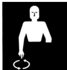
Figure 1.39 Lower the equipment. Use circular motion with either hand pointing to the ground. Example: Use this signal to have operator lower high lift or machine header.
