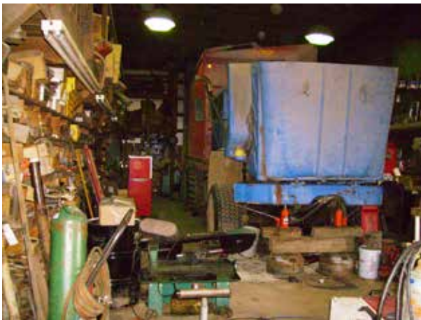
Figure 5.36 Sloppy housekeeping contributes to potential fire hazards in farm shops and other structures. What class or classes of fire (A, B, or C) could occur in the shop shown in the photo? Credit: J. Mathison.
