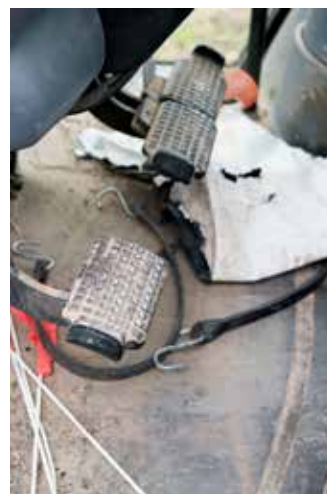
Figure 2.42 The operator's platform of a tractor is not a tool box. You must have room to operate hand and foot controls. PTO levers, differential locks, foot throttles, and brake locks have to be engaged from the floor position. Soda cans and tobacco snuff containers can roll under control pedals and prevent correct timely operation. Credit: J. Mathison.
