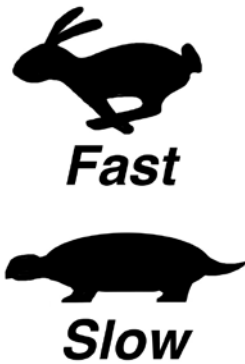
Figure 2.25 The throttle symbol reminds us of the slow turtle and fast rabbit story, or speed control. Credit: J. Mathison.
