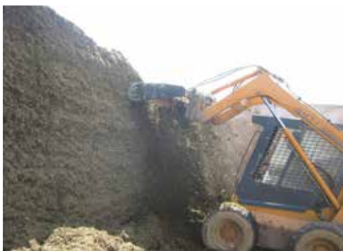
Figure 4.30 A hydraulic-powered, revolving-type silage defacer mounted to a skid-steer is used to evenly remove the silage from the entire feed-out face of the silage. The construction of the defacer allows the operator to view the task easily. Credit: J. Mathison.
