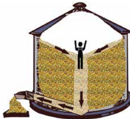
Figure 8.5 If a person stands on top of the grain while the unloading auger is running, grain flowing out of storage causes a downward-moving floor to move away from the person's feet. The victim is pulled waist deep in about 10 seconds. Credit: PSU Ag Safety.
