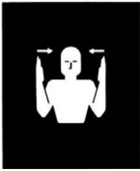
Figure 1.30 This far to go. Place palms at ear level facing head and move inward to show remaining distance to go. Example: Use this signal to assist a tractor operator in backing a loaded wagon or hitching to a wagon.
