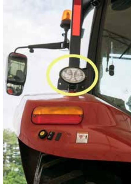
Figure 2.76 Be sure that a work light that points to the rear is off during road travel at night. Single white lights may not be recognized as slow-moving or as a tractor light. Credit: J. Mathison.
