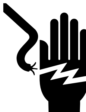
Figure 1.25 Potential electric shock hazard. Credit: Association of Equipment Manufacturers.
