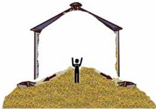
Figure 8.10 It takes much force to remove a grain bin entrapment victim. Rather than removing the victim, it is easier to remove the grain. Special tools and skills are needed to cut through grain bins and remove the grain. Credit: PSU Ag Safety.
