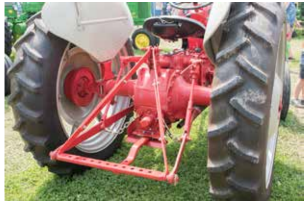
Figure 2.61 Hitch to the 3-point hitch drawbar. Credit: J. Mathison.
