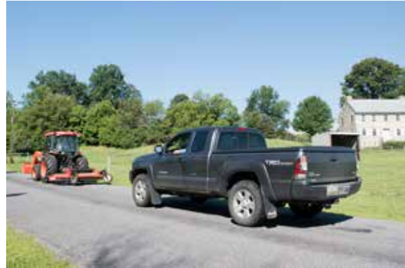
Figure 2.78 A best practice for transporting wide loads on a public roadway is to use an escort vehicle to assist in alerting other motorists. Be a courteous tractor operator to bring good public relations to the farm community. Credit: J. Mathison.
