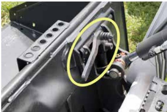
Figure 4.8 The standard latch handle lock for securing the attachment to the skid steer mounting plate is circled. The latch handle must be placed completely down to lock it in place. Credit: J. Mathison.
