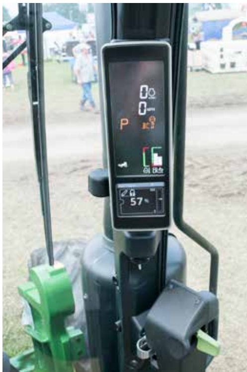
Figure 2.52 Visual monitoring of speed and power range assists the operator in efficient operation. Consult the operator's manual or ask your supervisor for directions so you can properly operate the tractor. Credit: J. Mathison.
