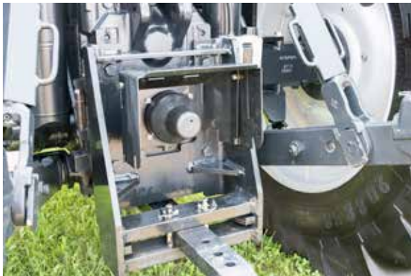
Figure 3.21 This PTO stub shaft is protected with a tractor master shield and stub shaft cover. To remove the stub shaft cover, grip the cover firmly and turn counterclockwise. Store the stub shaft cover where it will be available to replace when the job is done. Credit: J. Mathison.
