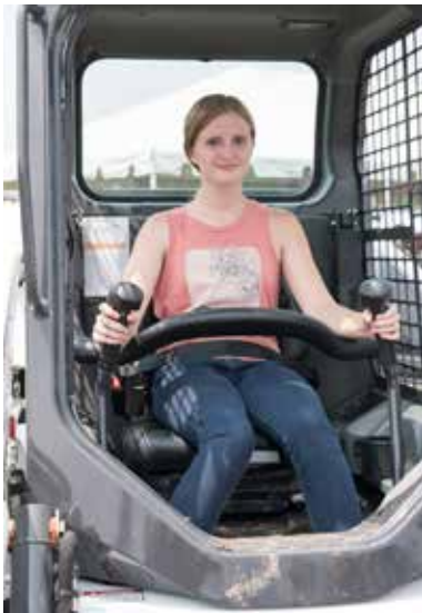
Figure 4.6 Control levers for moving or steering a skid steer are pushed forward, pulled back, or moved in some combination to “skid” the machine in the direction you wish to go. Notice the lap bar, which restrains the operator in the skid steer cab. Credit: J. Mathison.
