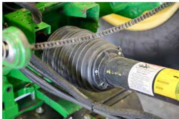
Figure 1.5 A properly guarded PTO will protect against the entanglement hazard. Credit: Central States Center for Agricultural Safety and Health.
