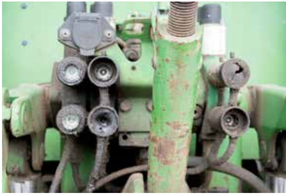
Figure 3.25 Missing hydraulic connection covers signify a problem with this tractor. What will happen to the hydraulic system if the dust covers are not kept in place? Credit: J. Mathison.
