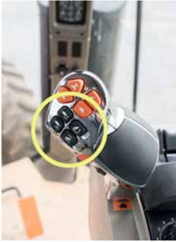
Figure 2.13 High lift controls are color-coded black. Credit: J. Mathison.
