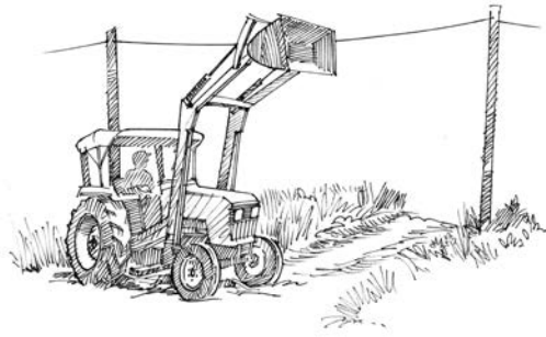
Figure 2.73 Be aware of overhead power lines while transporting equipment to avoid risk of electrocution. Credit: J. Mathison.
