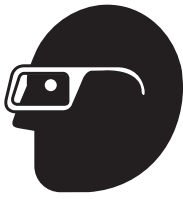
Figure 1.11 Industrial safety glasses are recommended when you see this symbol. They protect against flying and pointed projectiles and may come with brow and side-protection panels. Credit: Association of Equipment Manufacturers.
