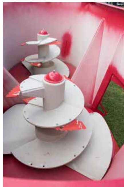
Figure 4.26 A total mix ration (TMR) mixing wagon loads from the top by high-lift bucket. This is not a normal work position and because of the distance away from the operator is considered to be guarded by location. DO NOT ENTER this mixing space, which has two augers moving close together. A hazard is guarded by location when it is guarded by other parts or components of the machine that are not themselves guards, or when the hazard is beyond the safety distance. The high sides of the mixing wagon form a barrier to prevent the hazardous area from being reached inadvertently. Credit: J. Mathison.
