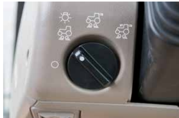
Figure 2.12 This switch depicts the various options for lighting on this tractor. Credit: J. Mathison.
