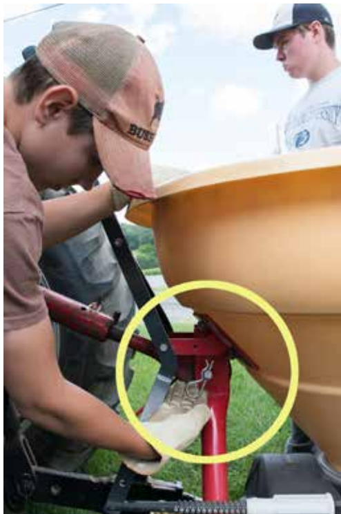
Figure 3.10 After adjusting the upper link of the tractor's 3-point hitch to align with the upper hitch point of the implement, secure the equipment with the proper size hitch pin and security clip. The circled area indicates where the upper link may be adjusted for fit. The implement must be in a level position after the connection is made. Credit: J. Mathison.
