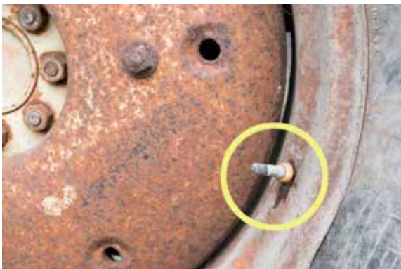
Figure 2.41 A leaking valve stem released calcium solution, which rusted the rim. A major expense would be incurred to replace the tire. There is also a severe safety hazard in using this tractor. Credit: J. Mathison.
