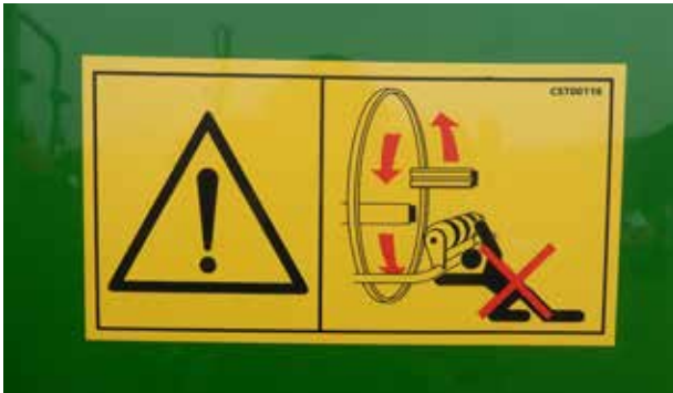
Figure 1.6 Pull-in points are found on harvesting machinery. This is a symbol for pull-in point hazard. Credit: Association of Equipment Manufacturers.
