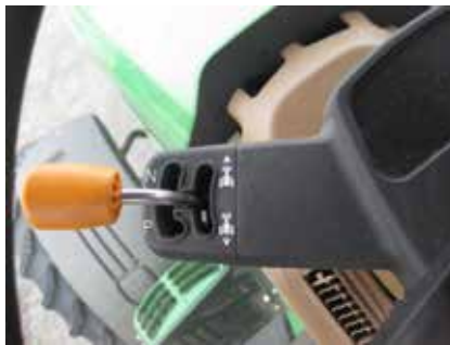
Figure 2.51 Look on the left side of the steering column. The shuttle shift lever, sometimes called the reverser, allows for ease of changing direction without using the clutch. This lever may serve as the positive park to be used with the parking brake. Some may have to be in a neutral position for the tractor to start. This may be the only time that the clutch pedal is used. Credit: J. Mathison.
