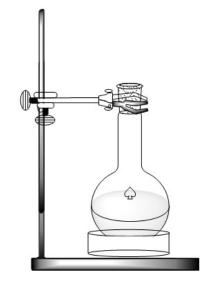
**Hazards:** Sulfur dioxide gas (SO<sub>2</sub>) is an irritant to lungs, throat, and eyes. In order to minimize SO<sub>2</sub> (g) exposure, perform this demonstration in a hood, or near an in-bench hood. If a hood is not available, get the burning sulfur into the flask as quickly as possible.
