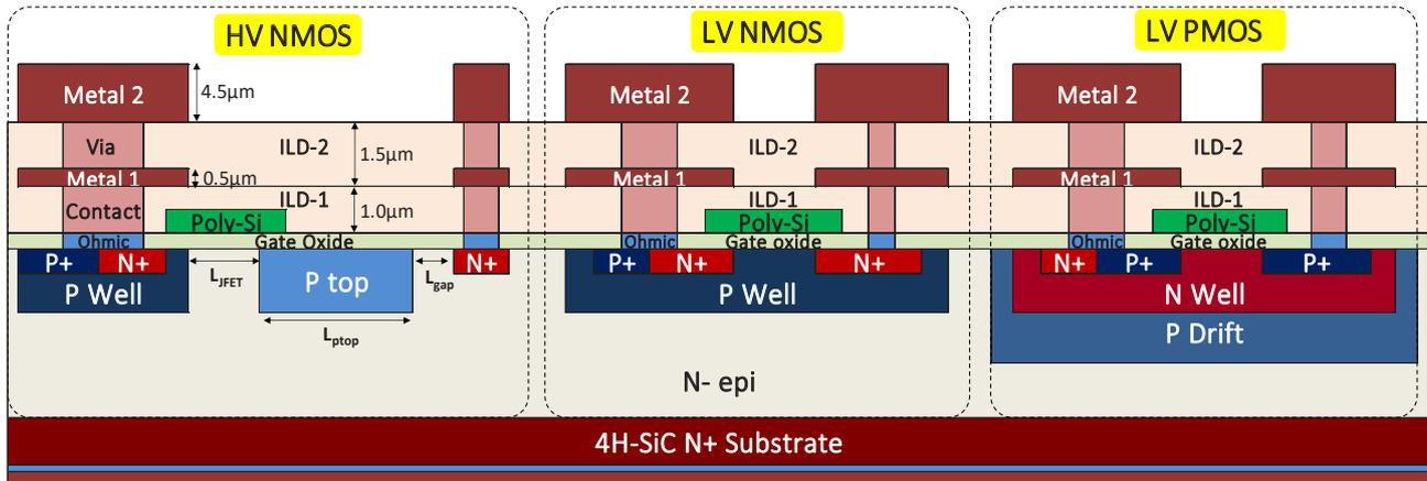
Figure 1: Cross-section of the fabricated HV NMOS, LV NMOS and LV PMOS on an N-epi grown on N+ substrate.
