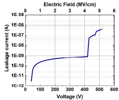
Figure 17: ILD breakdown across metal 1 and metal 2
