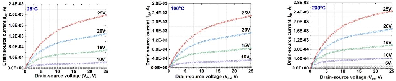
Figure 6: Output characteristics of 10  $\mu\text{m}$  wide, 1  $\mu\text{m}$  long LV NMOS at 25°C, 100°C and 200°C
