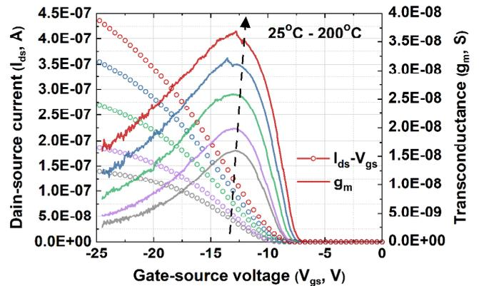
Figure 9: Transfer characteristics (at  $V_d=0.1$  V) of LV PMOS
