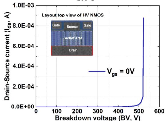
Figure 5: Blocking characteristics of HV NMOS measured at 25°C
