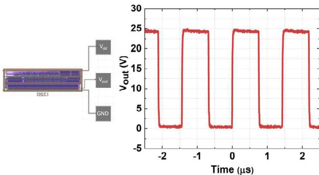
Figure 15: Layout view of CMOS ring oscillator and its operation for V<sub>dd</sub> of 25 V at 25°C
