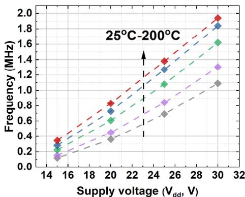
Figure 16: Ring oscillator frequency as a function of V<sub>dd</sub> over 25°C to 200°C
