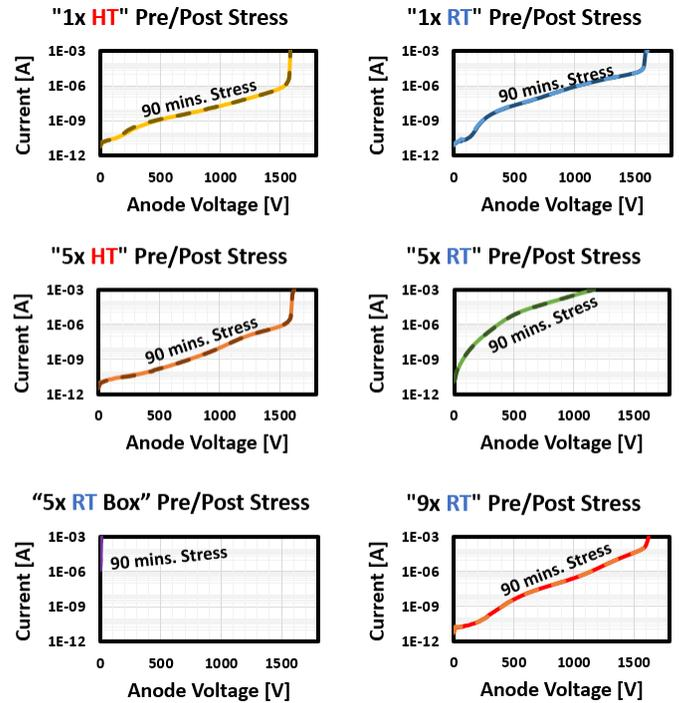
**Figure 12.** Comparison of reverse blocking behaviors of various JBS diodes pre (Solid) and post (Dashed) 125A/cm<sup>2</sup> current stress for 90 minutes. No change in the forward conduction can be observed following the current stress condition.
