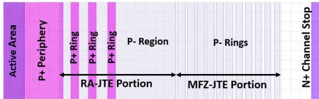
**Figure 3.** Design of the Hybrid JTE edge termination used to ensure near ideal breakdown voltage and minimal leakage current. Main components and P+ regions of the hybrid JTE edge termination are labeled. JTE and N+ regions were implanted at room temperature (25°C).
