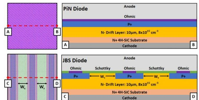
**Figure 1.** Top and cross sectional views of the 4H-SiC PiN Diode (top) and JBS Diode (bottom) used in this study. Optimal  $W_s$  for JBS diode was determined to be 2μm.
