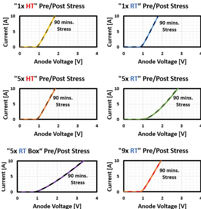
**Figure 11.** Comparison of forward IV curves of various JBS diodes pre (Solid) and post (Dashed) 125A/cm<sup>2</sup> current stress for 90 minutes. No change in the forward conduction can be observed following the current stress condition.
