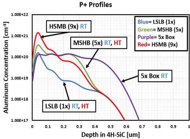
**Figure 2.** Aluminum concentration profiles used in the various P+ regions. All profiles were implanted at room temperature. LSLB (1x) and MSHB (5x) conditions were also implanted at high temperature of 600°C. Profiles were constructed using SRIM simulations.
