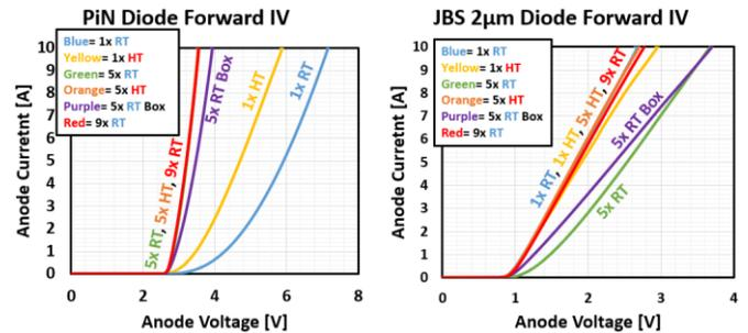
**Figure 6.** Typical forward IV performances of various PiN diodes (Left) and Nominal JBS diodes (Right). All IV characteristics were measured on wafer and at room temperature ( $25^\circ\text{C}$ ).
