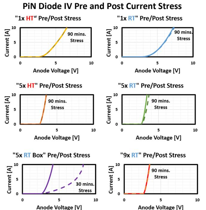
**Figure 9.** Comparison of forward IV curves of various PiN diodes pre (Solid) and post (Dashed) 125A/cm<sup>2</sup> current stress for 90 minutes with exception of the ‘5x RT Box’ condition which was halted after 30 minutes.
