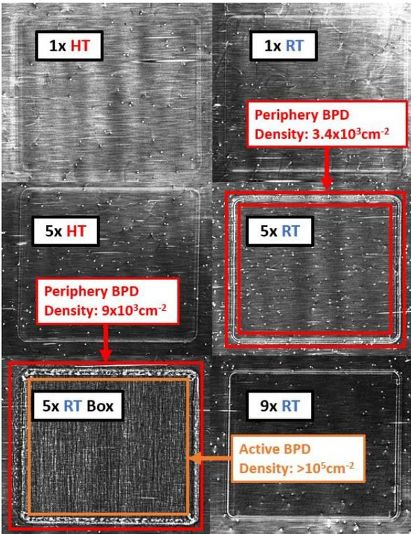
**Figure 5.** Post fabrication X-Ray topography images of the JBS diodes with various P+ implantation conditions. Areas of high BPD generation within the edge termination for the ‘5x RT’ and the ‘5x RT Box’ conditions, and active area for the ‘5x RT Box’ condition are highlighted in red and orange respectively.
