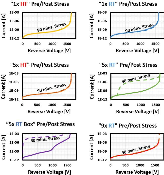
**Figure 10.** Comparison of reverse blocking behaviors of various PiN diodes pre (Solid) and post (Dashed) 125A/cm<sup>2</sup> current stress for 90 minutes with exception of the '5x RT Box' condition which was halted after 30 minutes.
