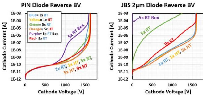
**Figure 8.** Typical blocking behaviors of various PiN diodes (Left) and Nominal JBS diodes (Right). All curves were measured on wafer and at room temperature (25°C).
