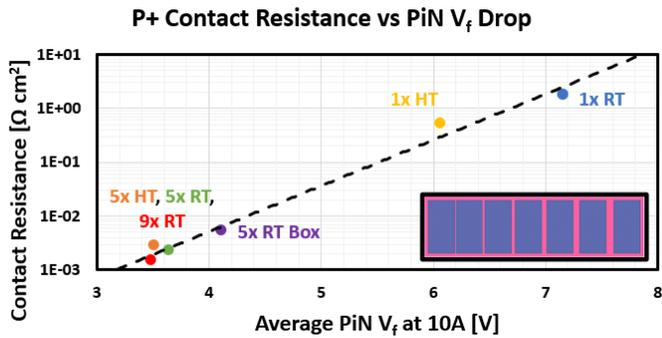
**Figure 7.** Correlation between the average PiN forward voltage drop at 10A for each P+ implantation condition and the average P+ contact resistance. Devices with higher surface doping concentrations contain lower resistance when compared to their lower surface concentration counterparts. Contact resistance was measured on wafer and at 25°C, using a bar type TLM structure.
