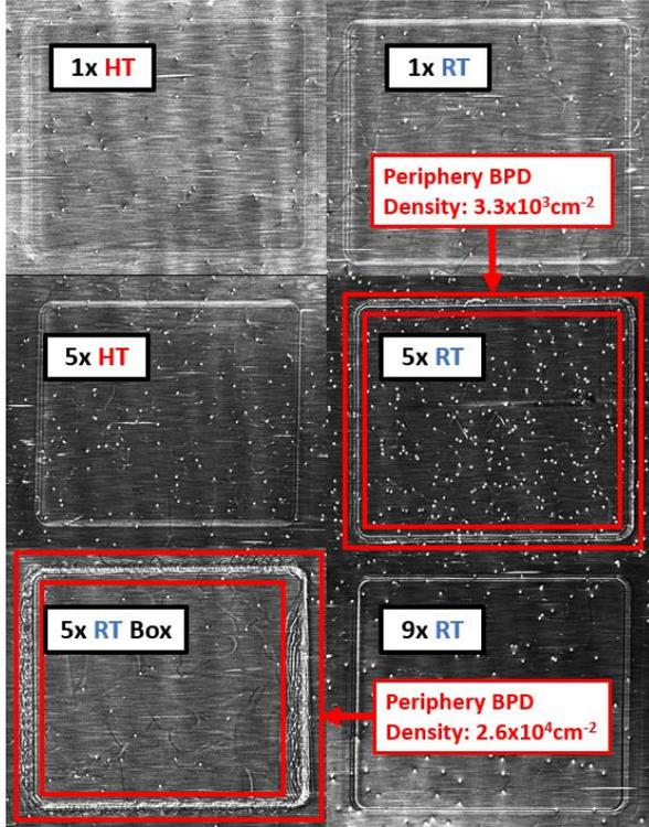
**Figure 4.** Post fabrication X-Ray topography images of the PiN diodes with various P+ implantation conditions. Areas of high BPD generation within the edge terminations for both the ‘5x RT’ and ‘5x RT Box’ conditions are highlighted in red.
