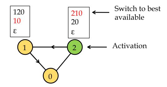
System is safe if all "fair" activation sequences lead to a stable path assignment
