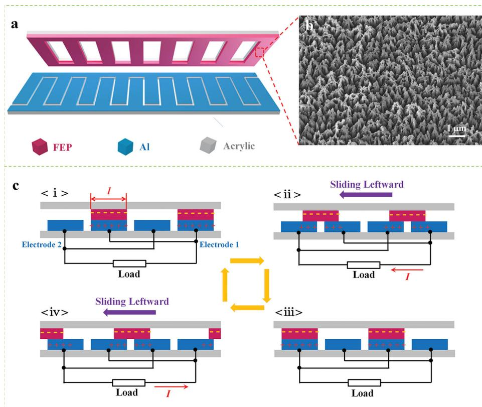
**Figure 1.** Device structure and operation mechanism of grating-structured freestanding triboelectric-layer nanogenerator (GF-TENG). (a) Typical structure design of GF-TENG. (b) SEM image of nanorod structure on the FEP surface. (c) Working mechanism of the GF-TENG.
