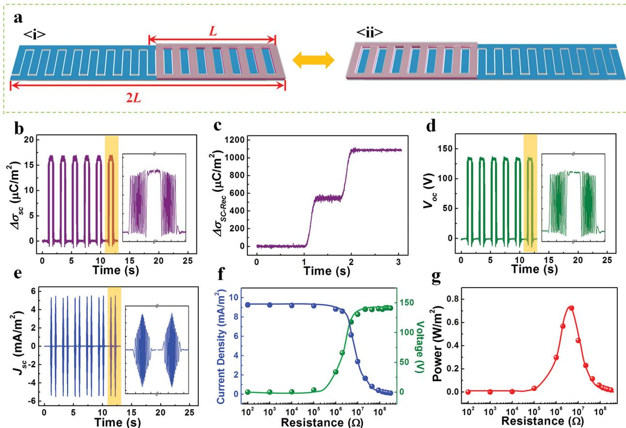
**Figure 4.** Electrical measurement results of the extended GF-TENGs. (a) The initial and final states of one-way sliding for a typical extended GF-TENG. (b–g) The measured results for the extended GF-TENG with 16 segments: (b) The  $\Delta\sigma_{SC}$ ; (c) The  $\Delta\sigma_{SC-Rec}$ ; (d) The  $V_{OC}$ ; (e) The  $J_{SC}$ ; (f) The dependence of the output voltage, current density, and (g) power density on the resistance of the external load.
