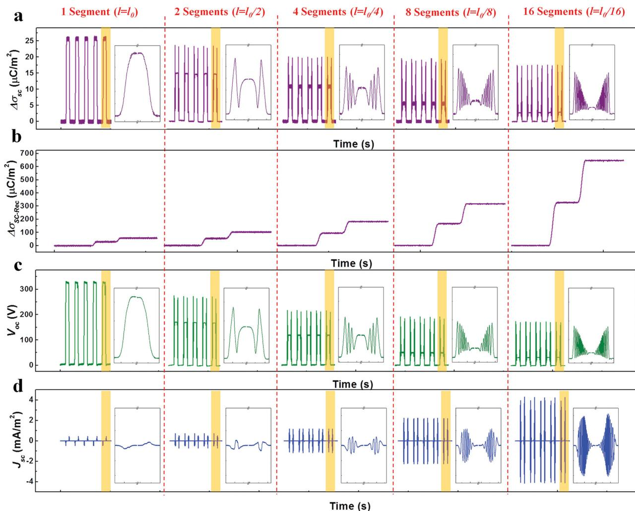
**Figure 3.** Electrical measurement results of GF-TENGs with different segment structures ( $N = 1, 2, 4, 8, 16$ ). (a) The measured  $\Delta\sigma_{SC}$ . (b) The measured  $\Delta\sigma_{SC-Rec}$ . (c) The measured  $V_{OC}$ . (d) The measured short-circuit current density ( $J_{SC}$ ). The insets show the enlargement of the corresponding highlighted parts.
