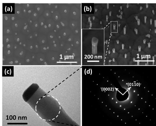
**Figure 1.** ZnO nanowires used for the reverse mode sample that were grown *via* a vapor–liquid–solid (VLS) deposition on a GaN epilayer: (a) top-down SEM image view; (b) SEM image at a tilt angle of 30° and a higher magnification image of a single nanowire (inset); (c) typical TEM image of a single ZnO NW with a gold droplet on its tip; (d) selected-area electron diffraction pattern from the region indicated by a dashed circle in image (c).
