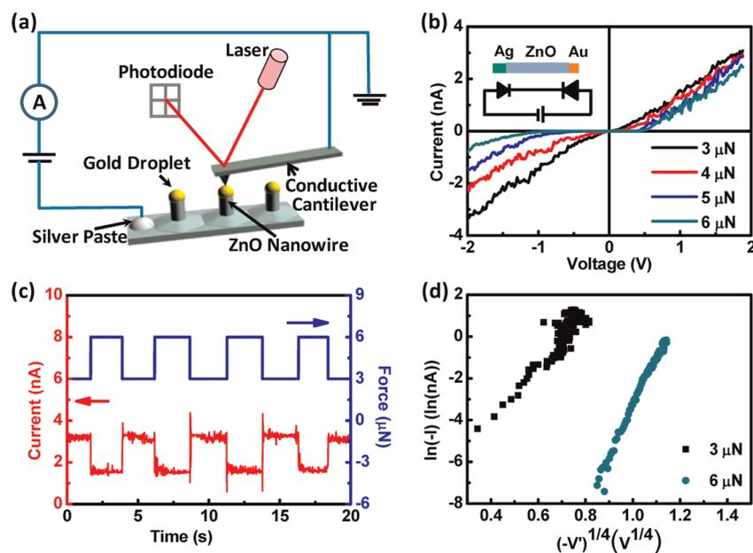
Figure 2. (a) Schematic of the conductive AFM system used for nanoscale positioning and electrical measurement; (b) typical  $I$ - $V$  characteristics under various compressive forces of a sample with double-Schottky junctions; (c) current response to a force pulse from 3 to 6  $\mu\text{N}$ ; the blue line is the applied force and the red is the resulting current; (d) plots of  $\ln(-I)$  as a function of  $(-V)^{1/4}$ , by using the data from the negative biased region in part (b).
