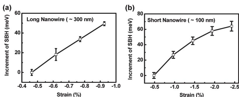
**Figure 5.** Schottky barrier increment with the strain at the Au–ZnO junction of a long nanowire device of  $\sim 300$  nm (a) and a short nanowire device of  $\sim 100$  nm and (b) calculated according to a thermionic emission–diffusion model.
