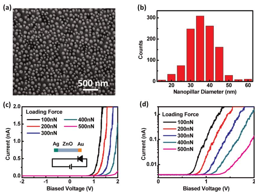
Figure 3. (a) ZnO nanowires used for the forward mode sample; (b) diameter distribution of the nanowires; (c)  $I$ – $V$  characteristics under various compressive forces of a sample with single-Schottky junctions; (d) current–voltage characteristics plotted on a semilogarithmic scale.
