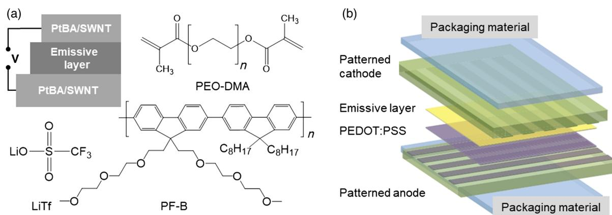
**Figure 4** | Fully stretchable LEEC devices. (a) The device structure of an LEEC based on an emission layer comprising PF-B, PEO-DMA, and LiTf, along with the chemical structures of these materials. Reproduced with permission from ref 42. Copyright 2011 Wiley-VCH. (b) Schematic illustrations of an encapsulated fully stretchable LEEC display. Reproduced with permission from ref 43. Copyright 2013 Springer Nature Limited.
