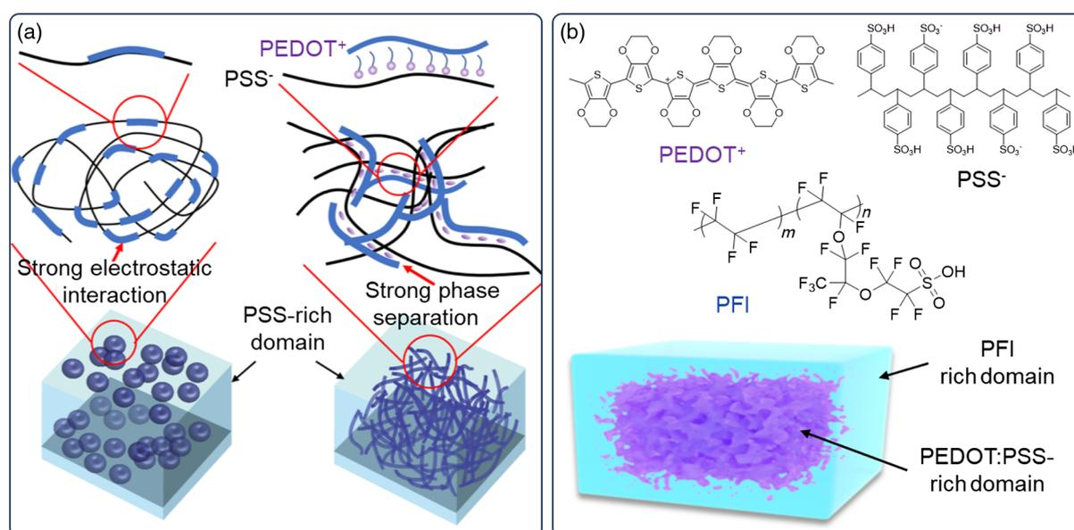
**Figure 12** | HTL/HIL for fully stretchable LED. (a) Schematics of the microstructures of pristine HTL and intrinsically stretchable HTL based on PEDOT:PSS\_Triton X composite. Reproduced with permission from ref 35. Copyright 2021 AAAS. (b) Chemical structures of PEDOT:PSS and PFI. Proposed 3D illustration of the morphology of the PEDOT:PSS\_PFI composite film. Reproduced with permission from ref 17. Copyright 2023, Springer Nature Limited.
