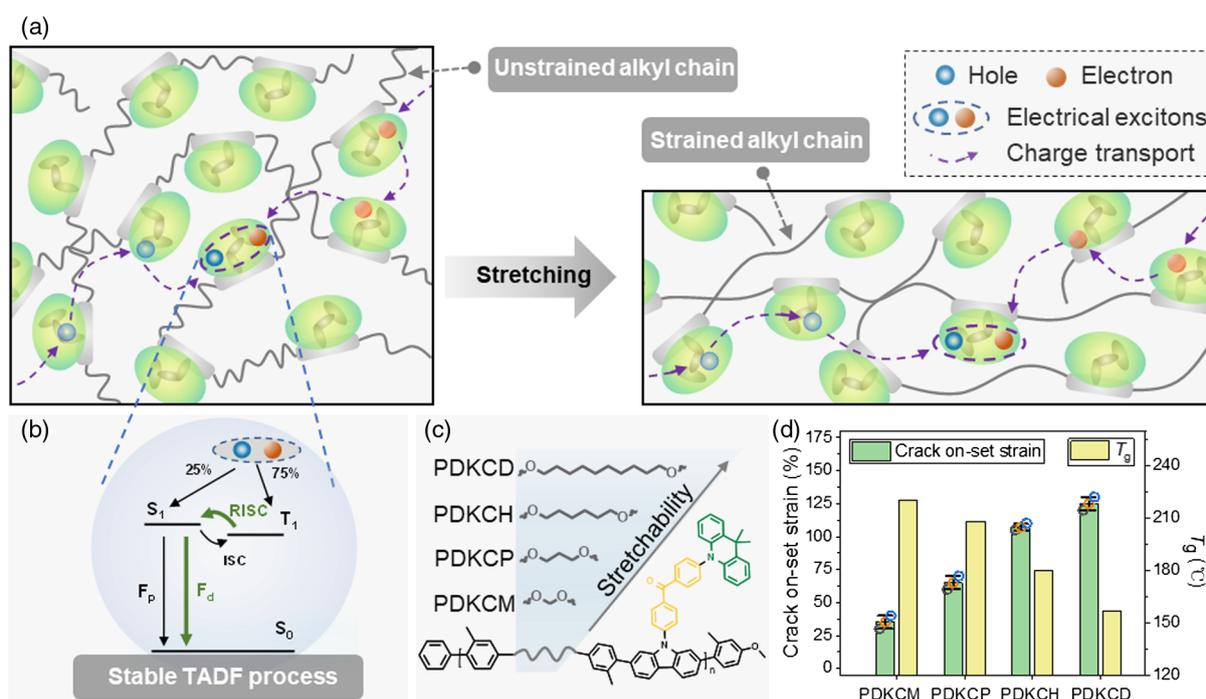
**Figure 10** | Intrinsic stretchable TADF-EMLs for LED. (a) Design principle for realizing stretchable TADF polymers via incorporation of soft alkyl chains into the polymer backbone. (b) Light-emitting mechanisms of the stretchable TADF polymer. (c) Chemical structures of stretchable TADF polymers having different alkyl chains in the polymer backbone. (d)  $T_g$  and crack onset strains of stretchable TADF polymers. Reproduced with permission from ref 17. Copyright 2023 Springer Nature Limited.
