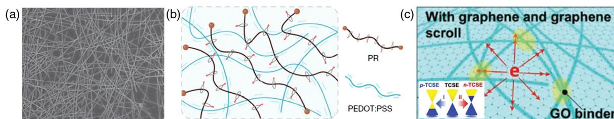
**Figure 11** | Stretchable electrode designs for fully stretchable LED. (a) SEM image of AgNW-PUA composite electrode. Reproduced with permission from ref 43. Copyright 2013 Springer Nature Limited. (b) Schematic morphology of a PEDOT:PSS/PR film. Reproduced with permission from ref 16. Copyright 2022 Springer Nature Limited. (c) Conceptual illustration of the fully stretchable OLED based on p- and n-doped TCSEs. Reproduced with permission from ref 87. Copyright 2022 Wiley-VCH.
