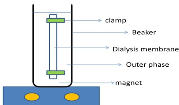
**Figure 2.1.** Schematic representation of *in vitro* release experimental system
