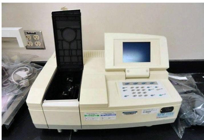
**Figure 2.2.** SHIMADZU UV-Visible 1700 spectrophotometer.
