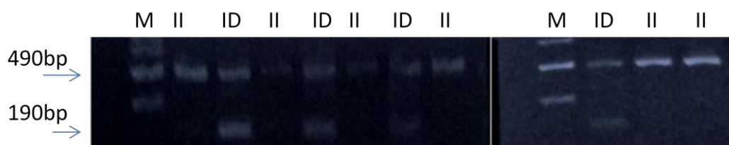
Figure 4.3 2% Agarose gel run at 85V 13 mA for 50 minutes. M demonstrates marker, 490bp insertion and 190 bp bands represents deletions
