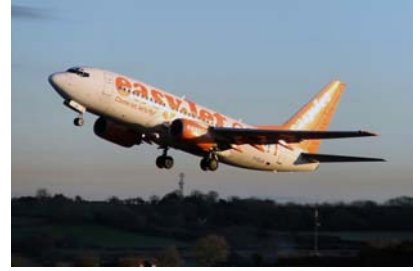
Figure C.11. Boeing 737-700: 30 kWh per 100 passenger-km. Photograph © Tom Collins.
