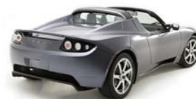
Figure 20.22. Tesla Roadster: 15 kWh per 100 km . www.teslamotors.com .
