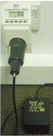
Figure 22.1. An awful AC lamp-adaptor from IKEA – the adaptor uses nearly 10 W even when the lamp is switched off!
