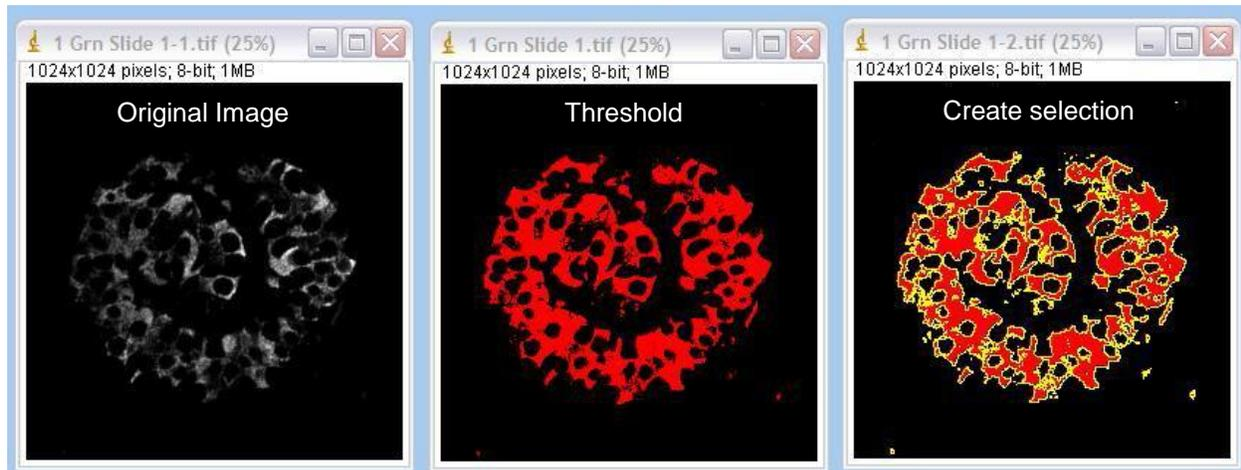
Once the object is thresholded, use Edit → Selection → Create Selection to outline the thresholded area. Finally, click the image you want to transfer the region to and use Edit → Selection → Restore Selection to create the region on the new image(s).
