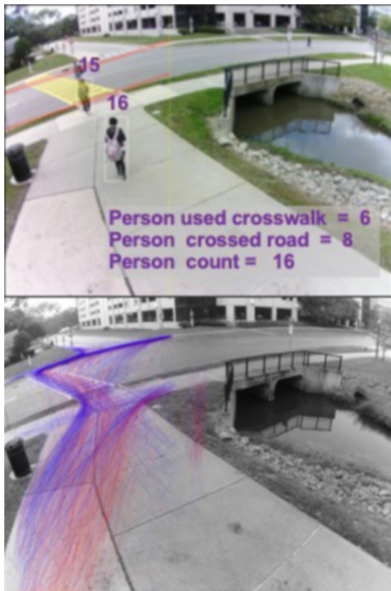
Fig. 4 Software-defined sensor to measure crosswalk usage. Images courtesy P. Bharti, D. Koop, and M. E. Papka, Northern Illinois University.
