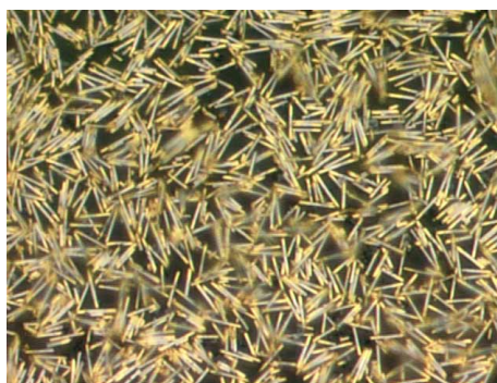
Figure 1: Optical micrograph of striped, Au, Pt, Au nanowires that are 200 nm in diameter and 5 microns long.
