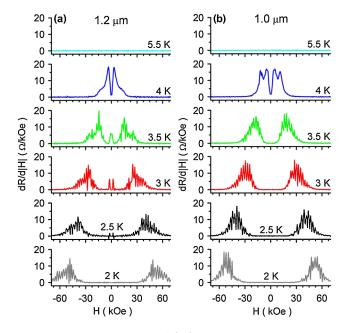
FIG. 3 (color online). dR/d|H| of the (a) 1.2  $\mu$ m and (b) 1.0  $\mu$ m Au nanowires.
