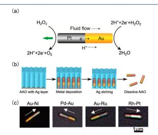
**Figure 1.** (a) Schematic of the self-electrophoretic propulsion of a Au–Pt bimetallic rod.<sup>1</sup> (b) Fabrication of metallic microrods by template-assisted electrodeposition.<sup>9</sup> (c) Examples of bimetallic rods of different combinations.<sup>15</sup> The direction of self-electrophoretic movement in  $H_2O_2$  is indicated by the arrow. Reproduced with permission from refs 1 and 15, Copyright 2012 and 2006 American Chemical Society; ref 9, Copyright 2013 Elsevier.
