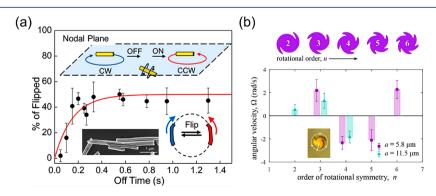
**Figure 5.** Shape asymmetry determines the directional motion of acoustic microswimmers. (a) Bent microrods orbit in the levitation plane.<sup>31</sup> (b) Twisted star-shaped microplates spin in clockwise or counterclockwise directions, depending on their chirality and number of arms.<sup>35</sup> Reproduced with permission from refs 31 and 35. Copyright 2017 and 2018 American Chemical Society.
