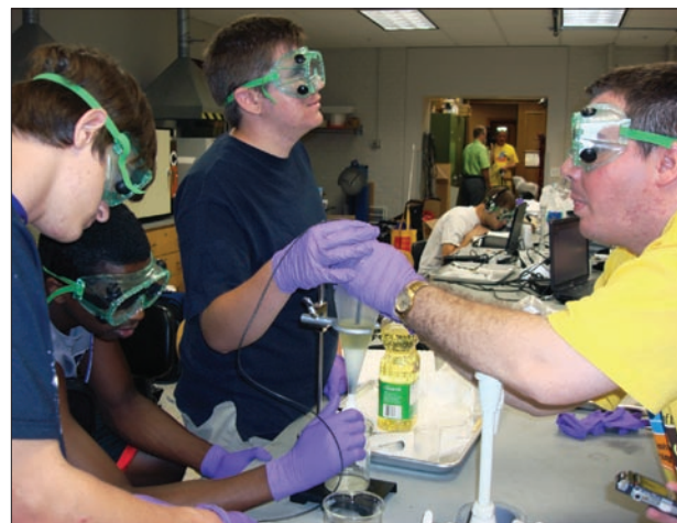
Figure 1. Teamwork is important as three students work with their mentor to detect the point at which the aqueous–organic meniscus passes the tip of the conductivity probe in the biodiesel experiment.
