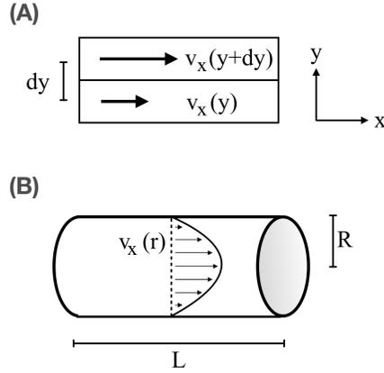
Figure 3: (A) Shear in the velocity gradient. (B) Parabolic laminar flow profile in a cylindrical pipe.
