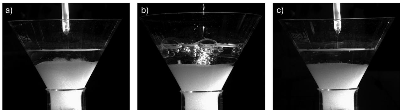
**FIG. 5.** Smaller jet diameter impact on dynamics. (a) Image of jet with halved diameter impacting bed at 2.5 cm above the bed. (b) Jet impacting bed at 22.5 cm above the bed. (c) Jet with lower flow velocity impacting bed at 2.5 cm above the bed. Multimedia available online.
