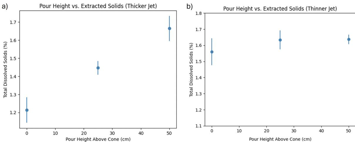
**FIG. 7.** Extraction experiments with real coffee. After making a pour-over using a Hario V60 cone, the resulting beverage is dried in the oven to determine the amount of contents extracted from the coffee grounds. (a) Total dissolved solids (%) against pour height in pour-over coffee using a higher and (b) lower flow rate from a gooseneck kettle, changing the radius of the jet.
