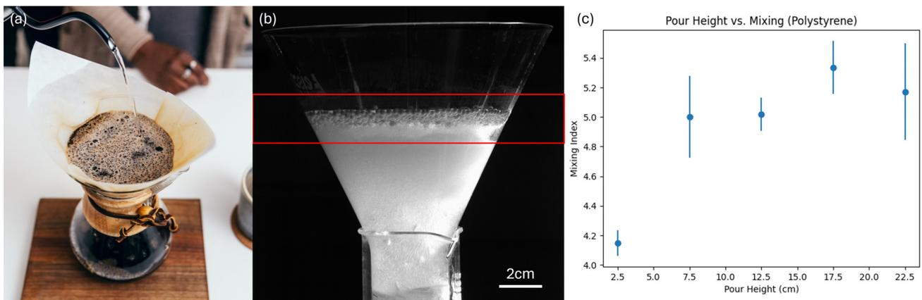
**FIG. 3.** Silica with floating polystyrene layer intensity vs height. (a) Image of a pour-over featuring many floating granules. Image by Matthew Henry, licensed under Burst Some Rights Reserved. (b) A floating polystyrene monolayer cast on top of the silica gel before the pour-over. (c) A plot of the mixing index vs pour height. Multimedia available online.
