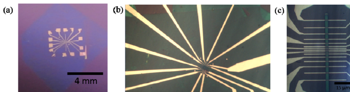
Figure S1. Graphene-hBN heterostructures. (a) Optical micrograph of electrodes in the TLM configuration contacting a graphene ribbon supported on five-layer CVD hBN. (b) Higher magnification optical micrograph of leads on five-layer hBN. (c) Optical image of PMMA etch mask (3 \mu\text{m} wide) spanning TLM design on a graphene-hBN stack.
