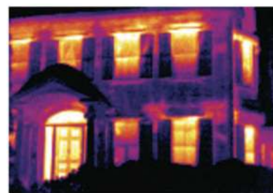
Figure 5.5: Thermal infrared image of a house in cold weather. The lighter regions are warmer and indicate areas with more heat loss, for instance due to missing insulation. From Introduction to Thermography Principles .
