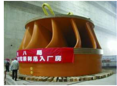
Figure 8.3: One of the 32 turbines installed in the Three Gorges Dam. Each generates 700 MW of electric power. Source: ???
