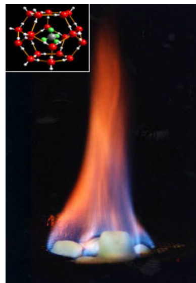
Figure 7.15: A molecular diagram of a methane hydrate clathrate in which water cages a methane molecule; and a picture of burning chunks of “ice,” which are really clathrate nodules. From the Naval Research Laboratory.
