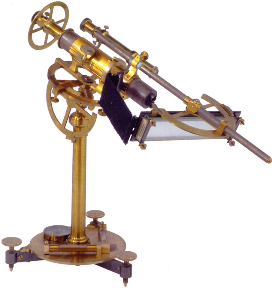
Fig. 3. Arago's cyano-polarimeter, built by Soleil © Collection École Polytechnique.
