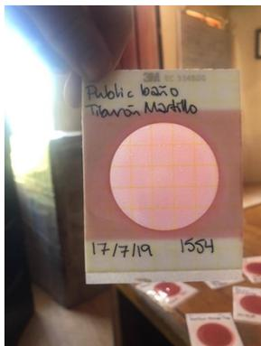
*Example of coliform test performed as part of the protocol.*
