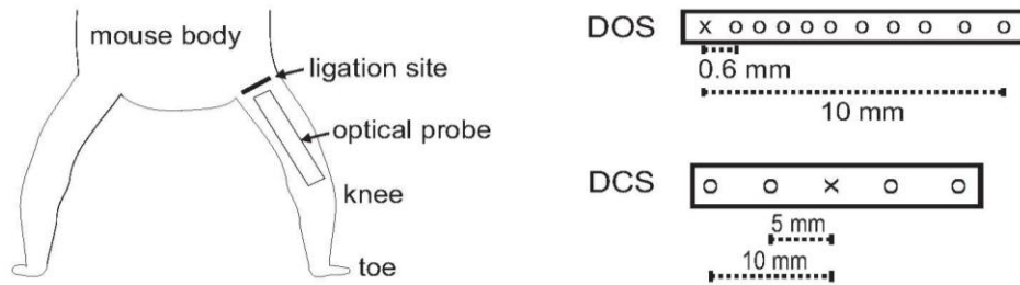
Fig. 1. Schematic diagram showing the position of the optical probe on the mouse hindlimb. The design of the probe is shown in the right side for both DOS (top) and DCS (bottom).
