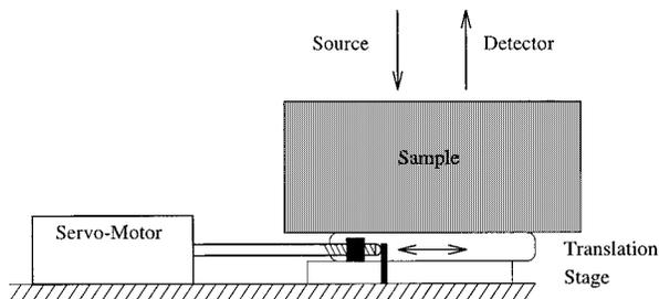
Fig. 5. Setup for performing the ensemble average.
